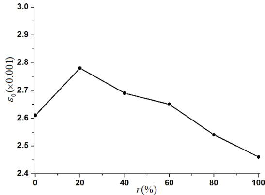
Fig. 6 Ultimate strain of glass fine aggregate concrete
