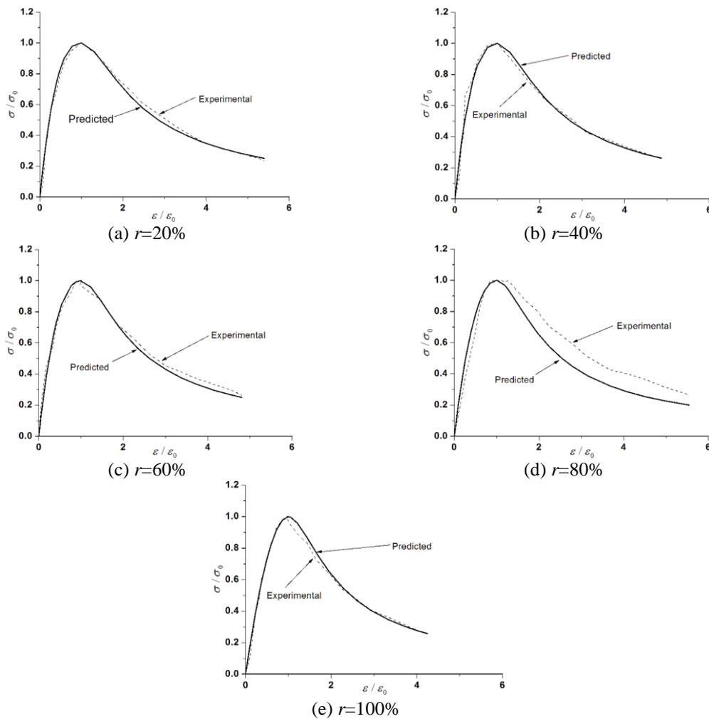
Fig. 7 Comparison of the normalized stress–strain curves
