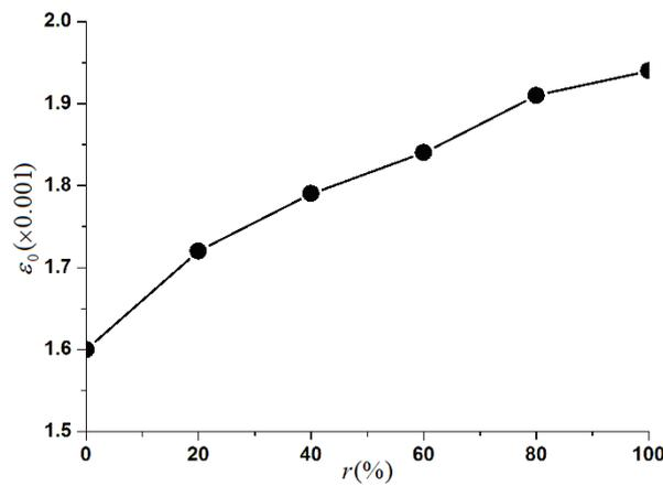
Fig. 4 Peak strain of glass fine aggregate concrete
