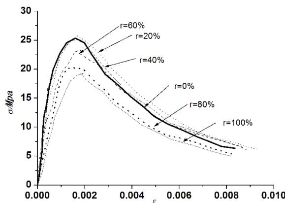
Fig. 3 Typical stress-strain curves of glass fine aggregate concrete
