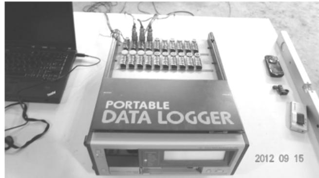
Fig. 5 The data logger used for measurement
