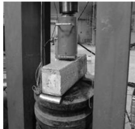
(a) Technical properties of concrete shear strength test machine and section (b) Devices made by the authors for testing the shear strength of concrete
