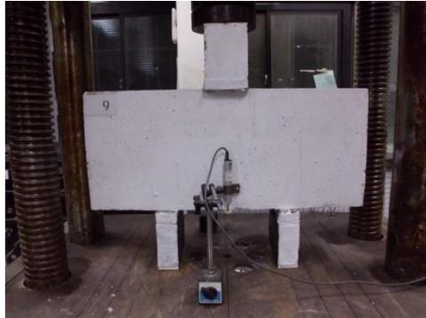
Fig. 2 Testing arrangements for deep beams
