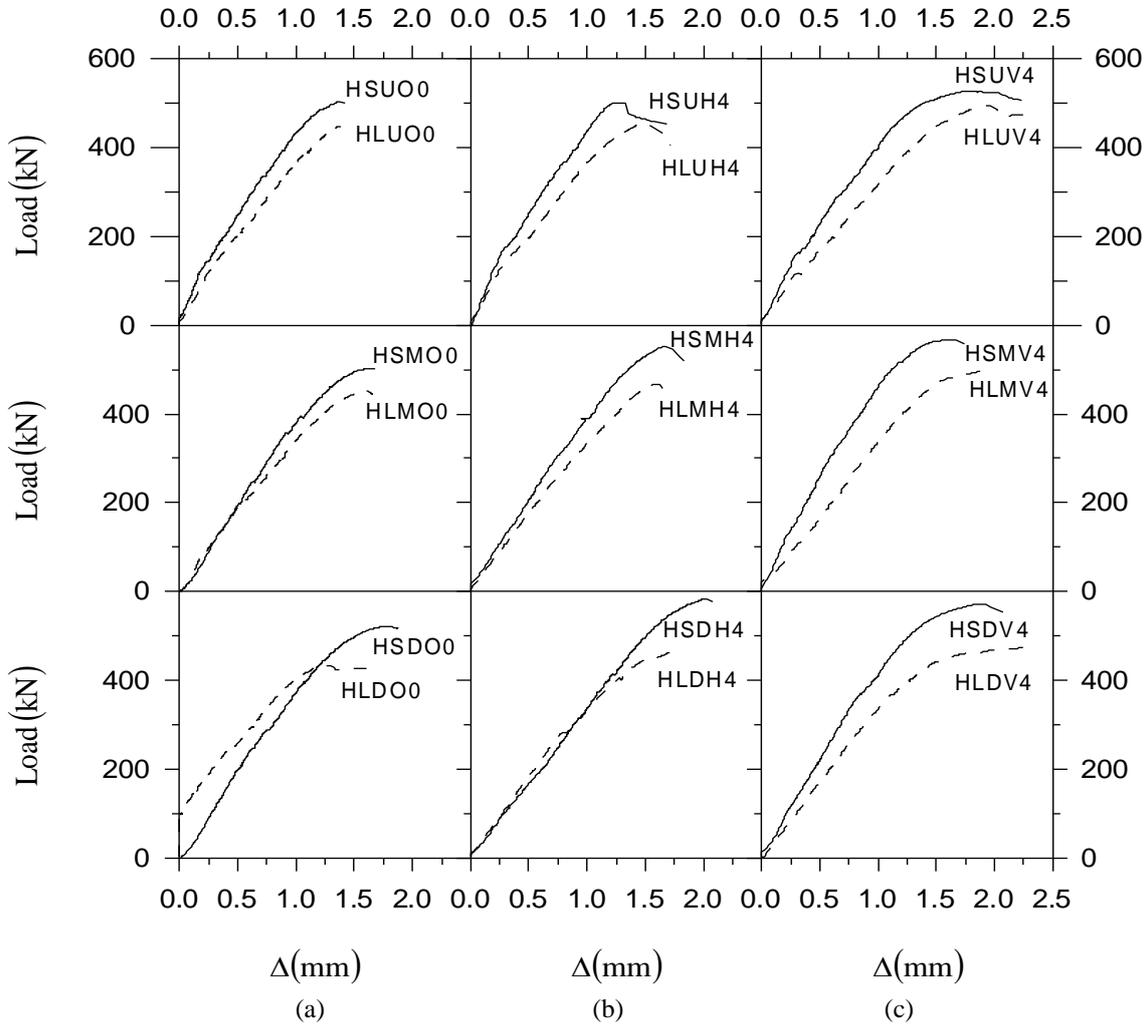
Fig. 4 Load plotted against displacement; (a) Not strengthened (b) Strengthened with CFRP in the horizontal direction (c) Strengthened with CFRP in the vertical direction
