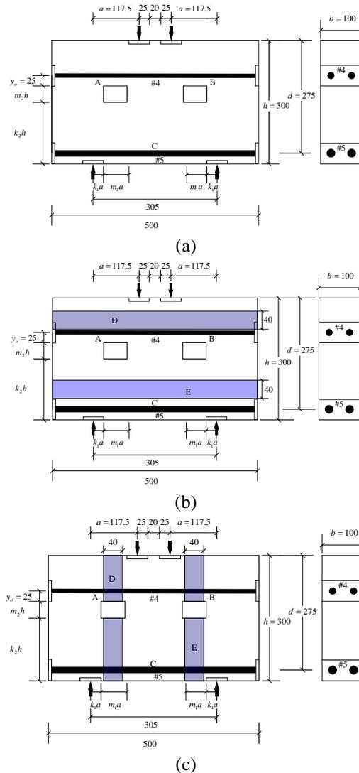
Fig. 1 Typical specimen; (a) Not strengthened (b) Strengthened with CFRP in the horizontal direction (c) Strengthened with CFRP in the vertical direction
