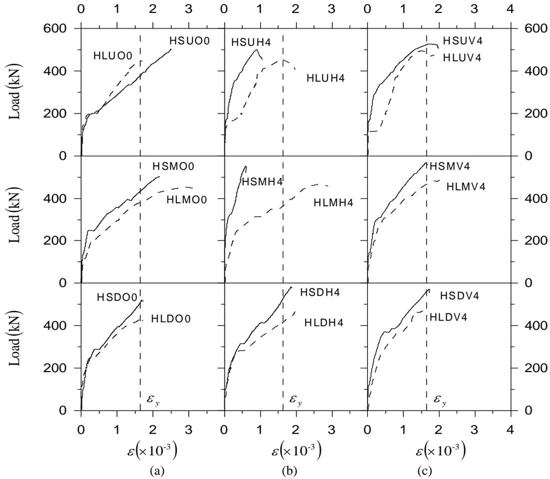
Fig. 5 Load versus strain of horizontal steels above the openings; (a) Not strengthened (b) Strengthened with CFRP in the horizontal direction (c) Strengthened with CFRP in the vertical direction
