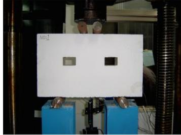
Fig. 2 Testing arrangements for deep beams
