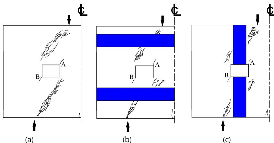
Fig. 3 Typical failure in deep beams tested; (a) Not strengthened (b) Strengthened with CFRP in the horizontal direction (c) Strengthened with CFRP in the vertical direction
