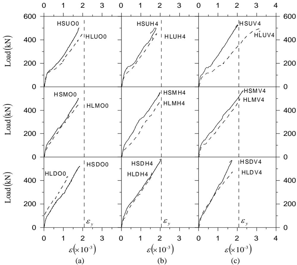
Fig. 6 Load versus strain of flexural steels; (a) Not strengthened (b) Strengthened with CFRP in the horizontal direction (c) Strengthened with CFRP in the vertical direction
