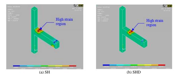
Fig. 12 Contour plots of third principal strain in concrete
