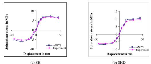
Fig. 10 Horizontal joint shear stress versus displacement curves
