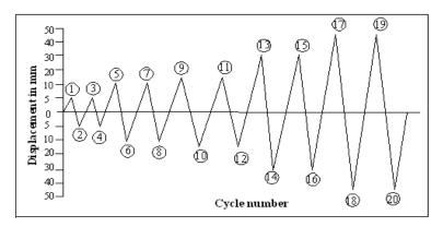
Fig. 4 Cyclic displacement loading
