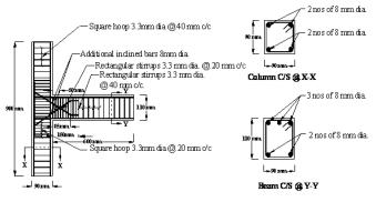
Fig. 2(b) Reinforcement details of SHD
