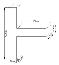
Fig. 1 Overall dimensions of test specimens
