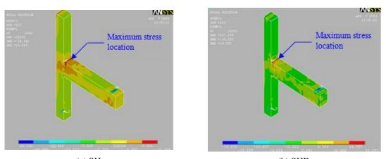
(a) SH (b) SHD Fig. 11 Contour plots of concrete first principal stress in concrete
