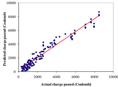
Fig. 4 Performance of the charge passed by nonlinear regression model
