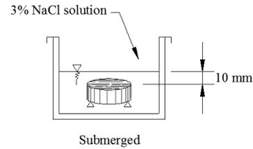
Fig. 2 Immersion of concrete specimen
