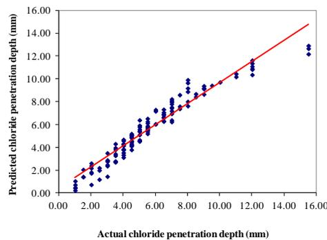
Fig. 5 Performance of the chloride penetration depth by nonlinear regression model
