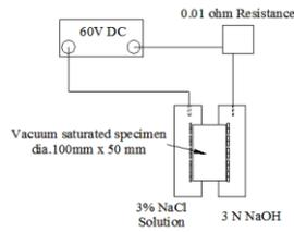
Fig. 1 Schematic diagram of RCPT test
