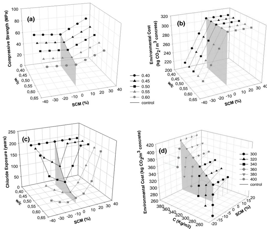
Fig. 5 Overall performance of SCM in terms of environmental cost (b), concrete strength (a) and service life properties (c) for a range of w/c ratios and for different initial cement content (d)
