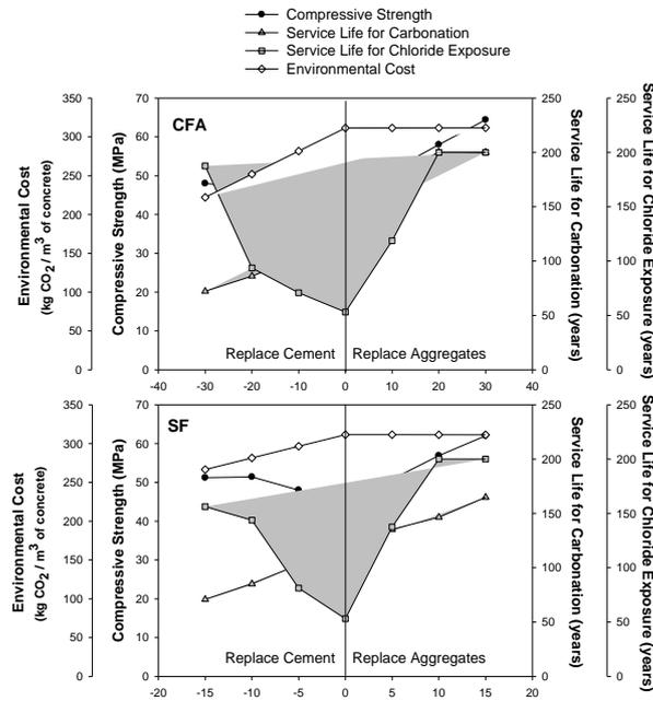
Fig. 4 Overall performance of CFA and SF mixes in terms of environmental cost, concrete strength and service life properties
