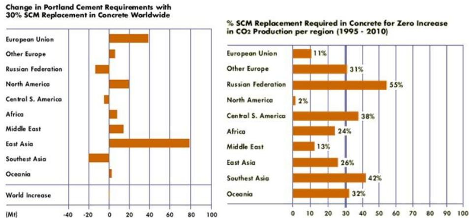
Fig. 1 Effect of SCM utilization in CO<sub>2</sub> emissions, after (Ecosmart concrete 2008)
