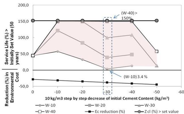
Fig. 9 Effect of reduction of water and cement contents on service life and environmental cost
