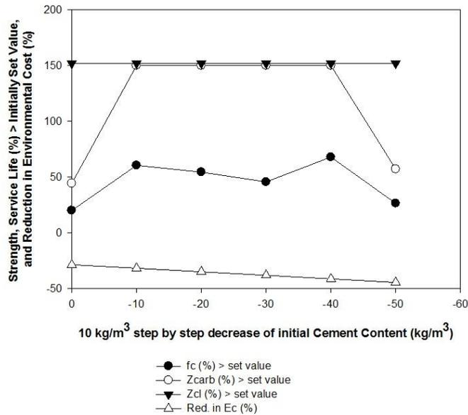
Fig. 7 Effect of step by step reduction of cement and water contents on the environmental cost and strength and service life values of a 30% CFA mix
