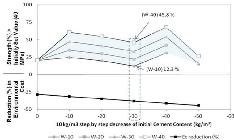
Fig. 8 Effect of reduction of water and cement contents on strength and environmental cost
