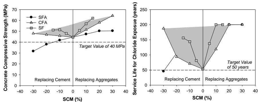
Fig. 3 Comparison of SF and FA performance in terms of target values for strength and service life
