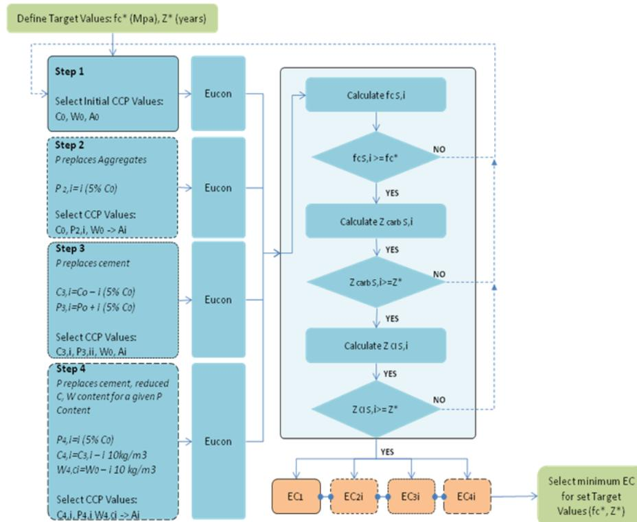
Fig. 2 Logical diagram of structured methodology for obtaining CCP values for minimum environmental cost (EC) with optimum strength and durability properties (C, P, W: cement, SCM and water contents, in kg/m<sup>3</sup>;  $Z_{carb}$ ,  $Z_{Cl}$ : service life in carbonation and chloride exposure, in years)
