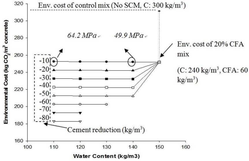
Fig. 6 Effect of step/step reduction of cement and water contents on the environmental cost of a 20% CFA mix
