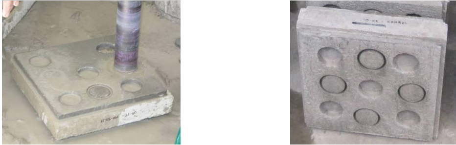
Fig. 7 Preparation of hole openings with a core driller after 6 months
