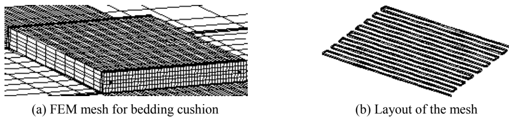
Fig. 26 Mesh for calculation
