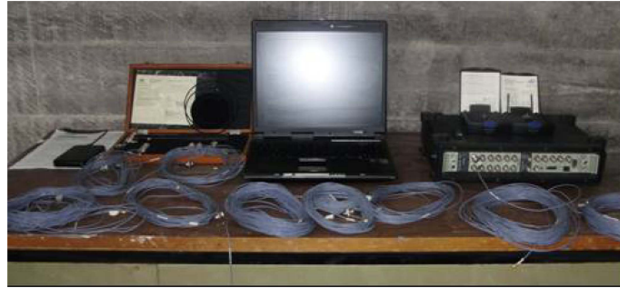
Fig. 4 Measurement equipment used for the ambient vibration tests
