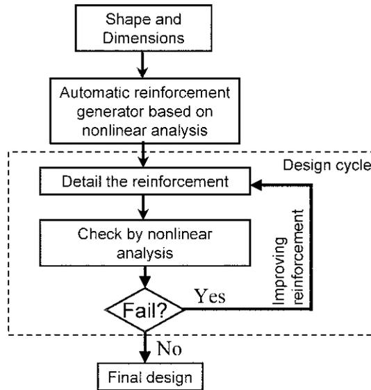
Fig. 9 Nonlinear analysis used also as a generator in the design process of RC structure
