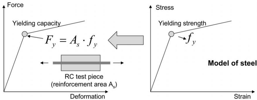
Fig. 3 Model of steel used for verification of yielding capacity of RC structure
