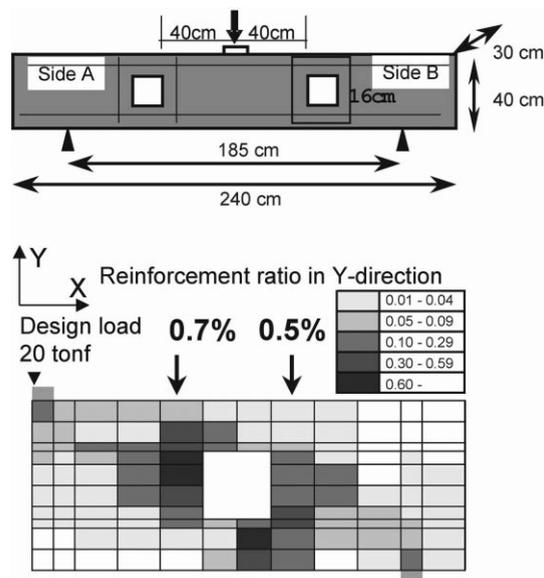
Fig. 10 Shape and dimensions of the beam and the output reinforcement ratio map (Y-direction)
