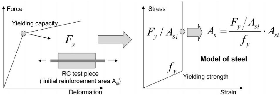
Fig. 4 Reversed process to decide steel amount from yielding capacity
