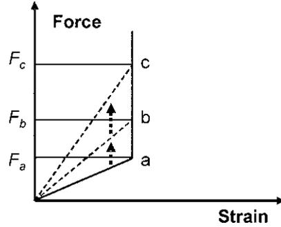
Fig. 5 A smart fictitious material model with strengthening behavior
