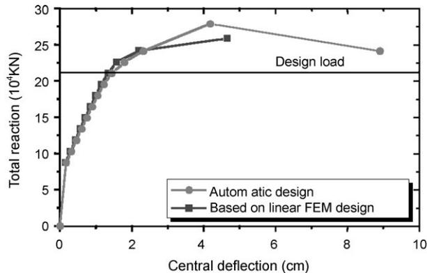
Fig. 20 Load-deflection results from the nonlinear FEM analysis (CASE31)
