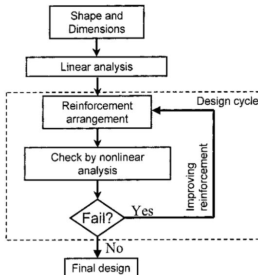
Fig. 1 Nonlinear analysis used as a checker in the design process of RC structure
