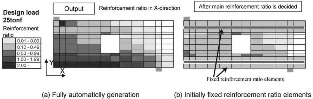
Fig. 7 Two kinds of reinforcement ratio map (X-direction) generated for design load
