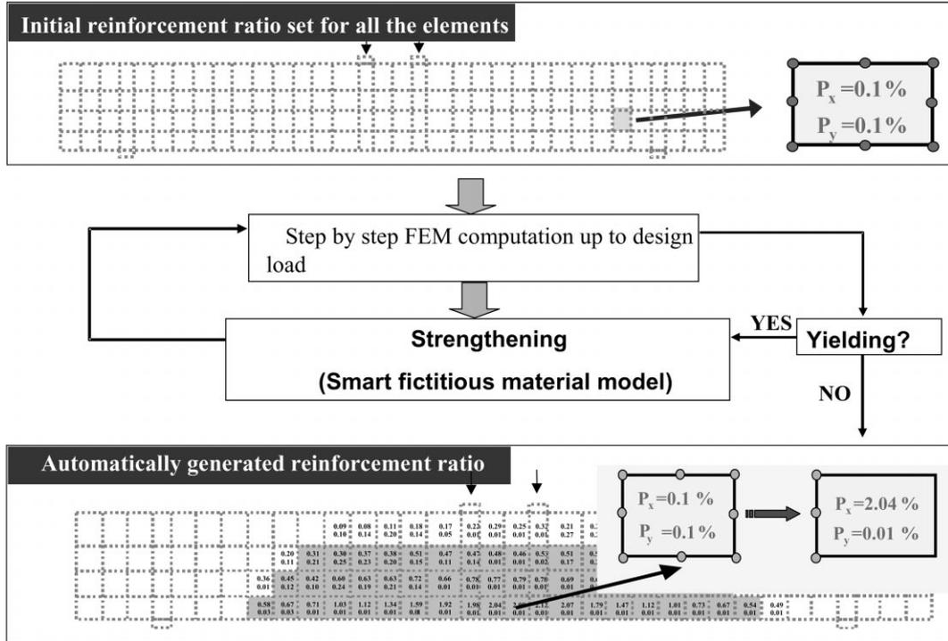
Fig. 6 Flow chart for automatically generating of reinforcement ratio in RC structures
