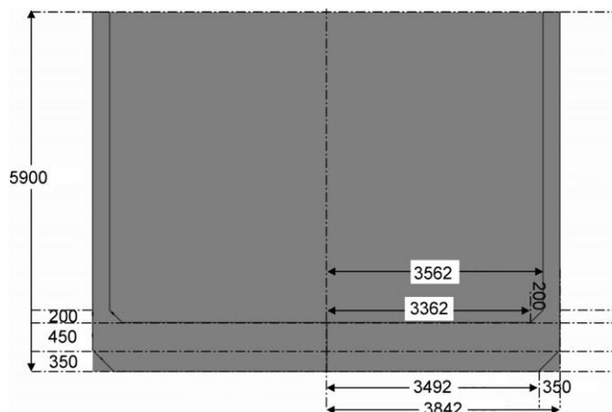
Fig. 16 Shape and scale of a LNG tank (Axial section, unit: cm)
