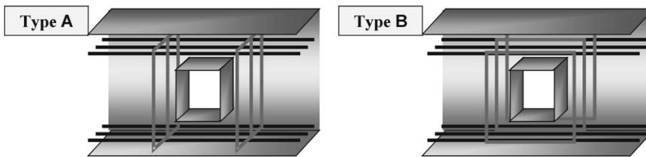
Fig. 11 Two types of shear reinforcing bars used to strengthen the opening
