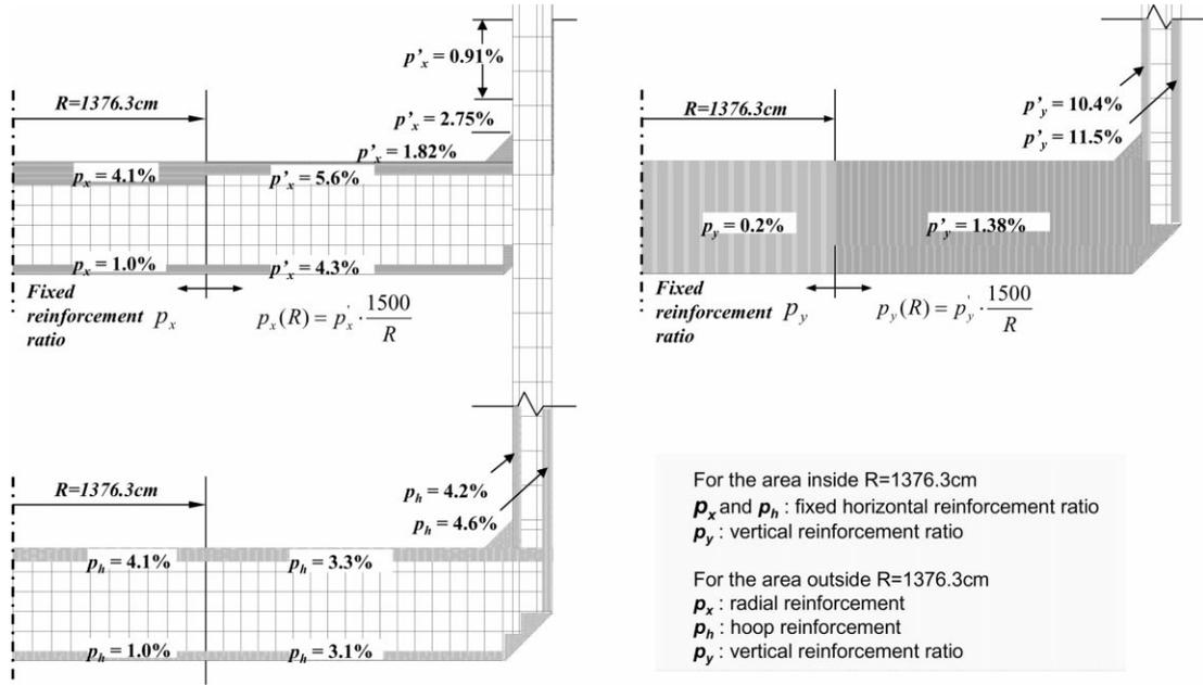
Fig. 19 Proposed reinforcement ratio based on the linear FEM analysis
