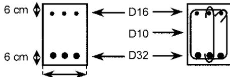
Fig. 12 Detail of reinforcement (Side A)
