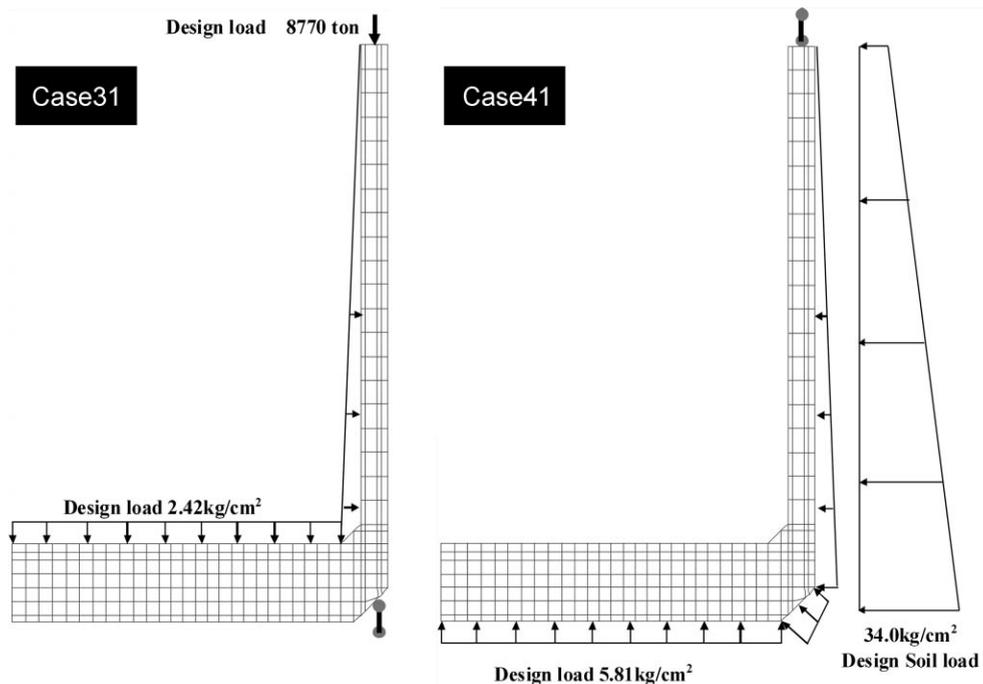
Fig. 17 FEM computation model and design loading cases of the LNG tank
