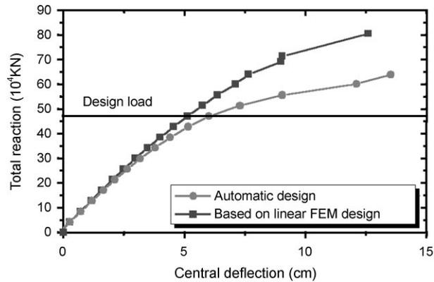
Fig. 23 Load-deflection results from the nonlinear FEM analysis (CASE41)
