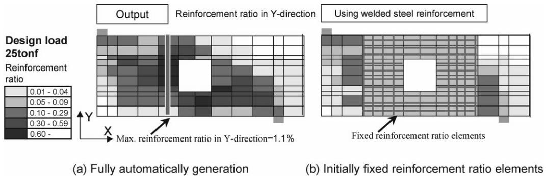
Fig. 8 Two kinds of reinforcement ratio map (Y-direction) generated for design load
