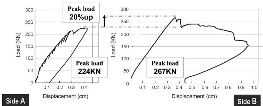
Fig. 14 Load-deflection (center) relationship of the beam
