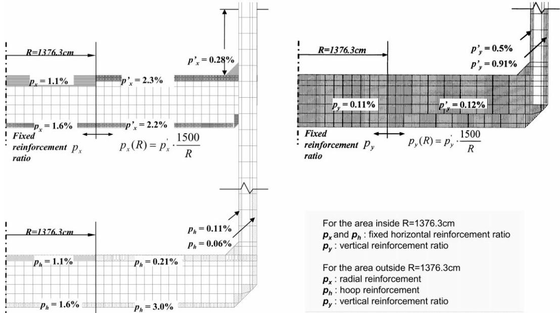
Fig. 18 Proposed reinforcement ratio based on the automatically computed results
