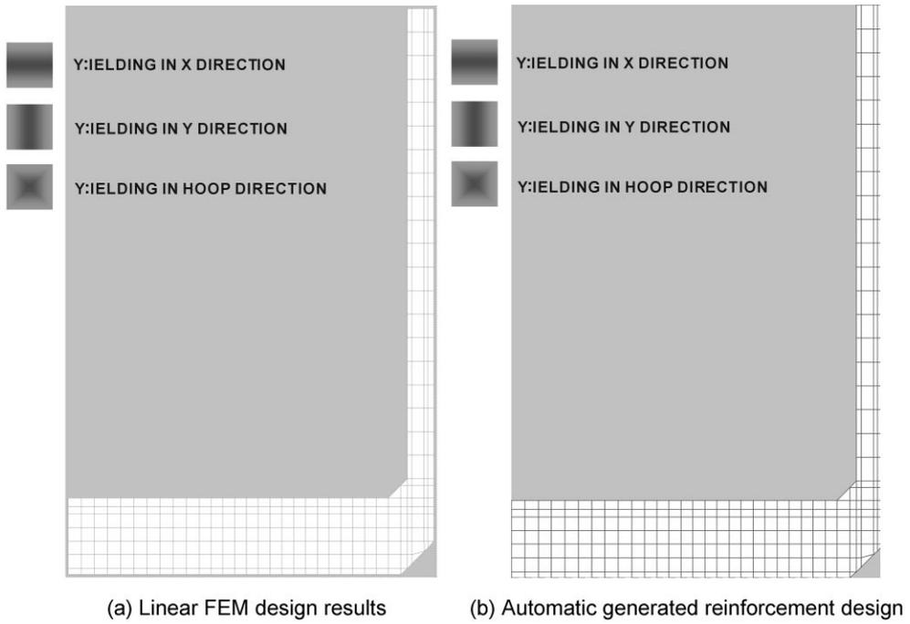
Fig. 21 Yielding map of reinforcement at design loading of Case31
