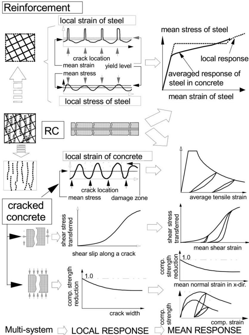
Fig. 2 Constitutive models for RC in a nonlinear FEM program
