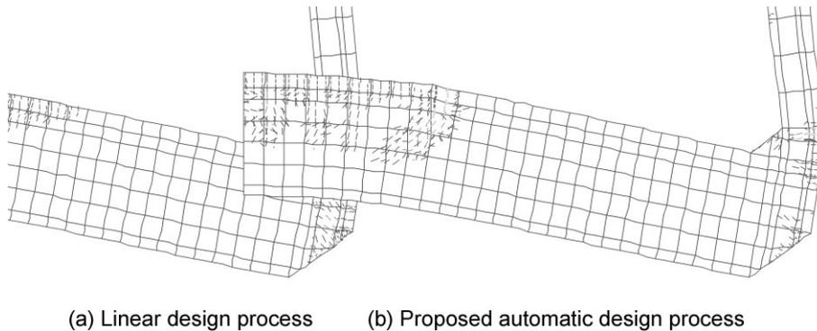
Fig. 25 Zoom up of crack patterns at the corner of LNG tank at failure stage (Case41)
