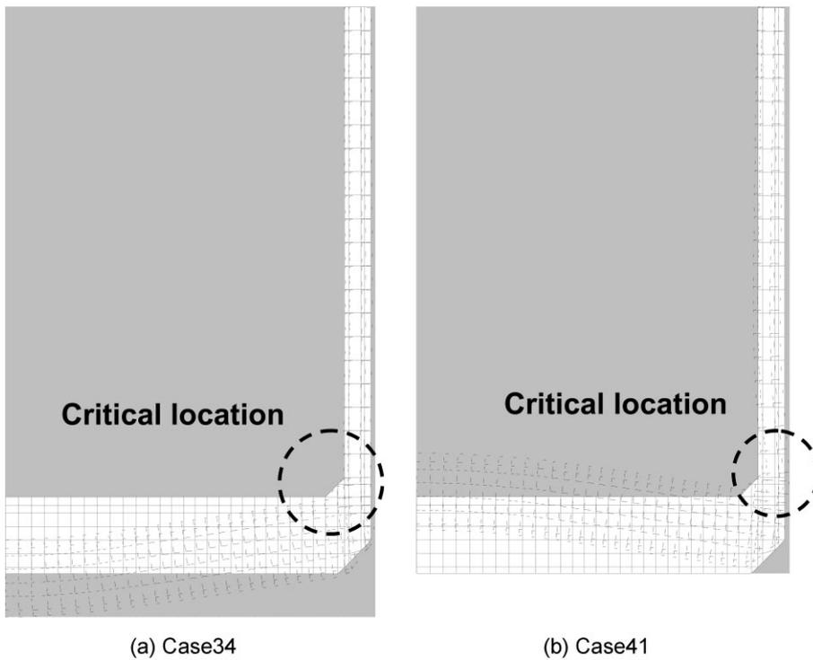
Fig. 22 Typical deformation and critical location of the RC LNG tank
