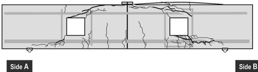
Fig. 15 Crack patterns for two sides of the beam
