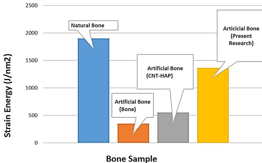
Fig. 6 Compression of strain energies between the introduced bone scaffold with a 1% carbon nanotube volume fraction with two phase bone scaffolds, common metallic artificial bone and with the natural bone (PourAkbar Saffar *et al.* 2010, Jamilpour *et al.* 2011)
