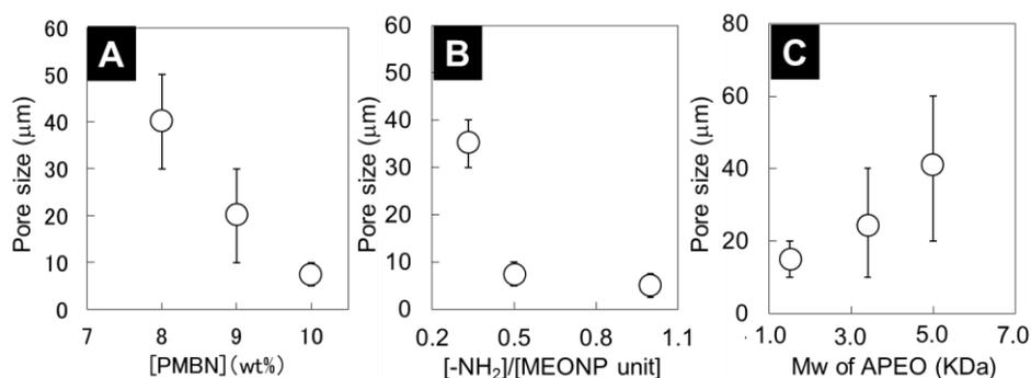
Fig. 8 Parameters affecting the pore size of the PMBN hydrogel cross-linked with APEO. Gelation was carried out at 37°C. Pore size of the PMBN hydrogels depended on [PMBN] (a),  $[-NH_2]/[MEONP \text{ unit}]$  (b), and Mw of APEO (c)
