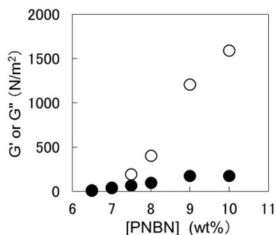
Fig. 4 PMBN concentration dependence on G' and G'' of PMBN hydrogels cross-linked with APEO. The reaction was carried out at 37°C. Open circle: G' elastic modulus; closed circle: G'' loss modulus
