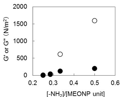
Fig. 5 [-NH<sub>2</sub>]/[MEONP unit] ratio dependence on G' and G'' of PMBN hydrogel cross-linked with APEO. Reaction was carried out at 37°C. Open circle: G' elastic modulus; closed circle: G'' loss modulus
