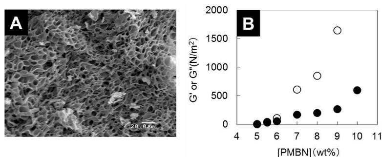
Fig. 7 (a) SEM pictures of PMBN hydrogel cross-linked with APEO ( $M_w=1.5 \times 10^3$ ) [PMBN]=8 wt%  $[-NH_2]/[MEONP \text{ unit}]=0.50$ , and (b) mechanical properties of the PMBN hydrogel with various concentrations of PMBN and  $[-NH_2]/[MEONP \text{ unit}]=0.50$ . The cross-linking reaction was carried out at 60°C. Open circle: G' elastic modulus; closed circle: G'' loss modulus
