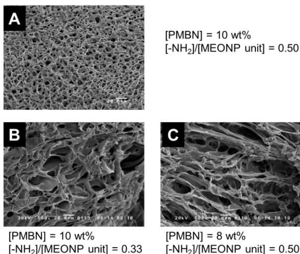
Fig. 6 SEM pictures of PMBN hydrogel cross-linked with APEO ( $M_w=1.5 \times 10^3$ ). Cross-linking reaction was carried out at 37°C. a: [PMBN]=10 wt%, [-NH<sub>2</sub>]/[MEONP unit]=0.50; b: [PMBN]=10 wt%, [-NH<sub>2</sub>]/[MEONP unit]=0.33; c: [PMBN]=8 wt%, [-NH<sub>2</sub>]/[MEONP unit]=0.50
