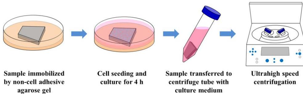
Fig. 1 Illustration of cell seeding on a Ti sample immobilized by non-adhesive agarose gel and the subsequent centrifugation process
