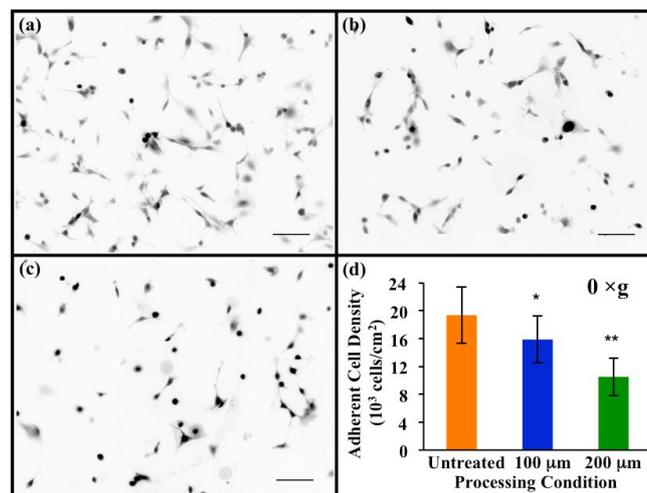
Fig. 2 Representative images of adherent cells on (a) untreated, (b) 100  $\mu\text{m}$  laser treated, and (c) 200  $\mu\text{m}$  treated Ti samples without centrifugation (scale bar: 100  $\mu\text{m}$ ); (d) the density of adherent cells on different substrates without centrifugation. (\* and \*\* denote statistical differences at  $p < 0.05$  compared to untreated and 100- $\mu\text{m}$ -spacing treated substrates, respectively)
