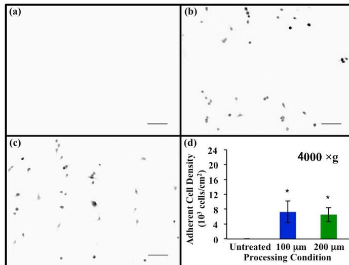
Fig. 4 Representative images of adherent cells on (a) untreated, (b) 100 μm laser treated, and (c) 200 μm treated Ti samples after 4,000 ×g force centrifugation (scale bar: 100 μm); (d) the density of adherent cells on different substrates after centrifugation at 4,000×g. (\* denotes statistical differences at  $p < 0.05$  compared to untreated substrates)
