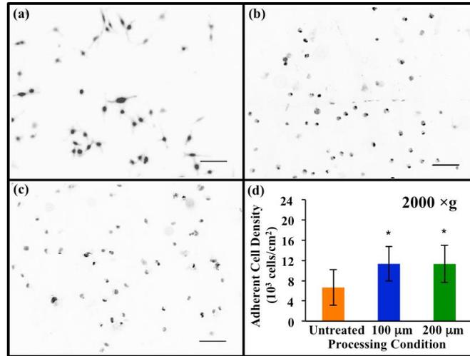
Fig. 3 Representative images of adherent cells on (a) untreated, (b) 100 μm laser treated, and (c) 200 μm treated Ti samples after 2,000 ×g force centrifugation (scale bar: 100 μm); (d) the density of adherent cells on different substrates after centrifugation at 2,000×g. (\* denotes statistical differences at  $p < 0.05$  compared to untreated substrates)
