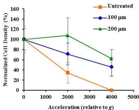
Fig. 5 Remaining fraction of adherent cells on different substrates as a function of centrifugation forces (results presented as the percentages to the cell density on non-centrifuged sample for each group)
