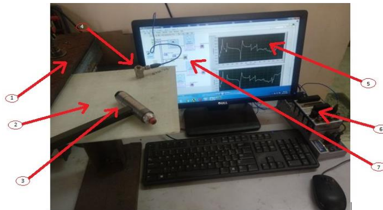
1. Fixture 2. Cenosphere Glass-epoxy composite 3. Impact hammer 4. Accelerometer 5. Output window 6. cDAQ 7. Block diagram of the LABVIEW
