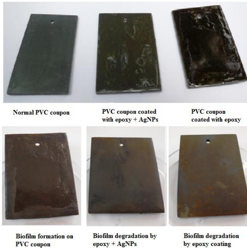
Fig. 8 PVC coupons with epoxy coating and Silver nanoparticles mediated epoxy coating on PVC materials and its anti-scaling (biofilm) activity
