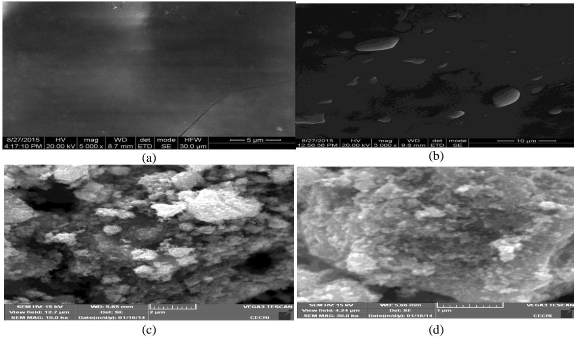
Fig. 3 SEM micrographs showing (a) PVC coupon, (b) epoxy coated PVC coupon and (c), (d) epoxy coated with silver nanoparticles
