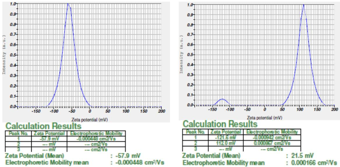
Fig. 7 Dynamic light scattering analysis (a) Zeta potential of *Alstonia scholaris* mediated synthesis of AgNPs (b) Zeta potential of epoxy coated *Alstonia scholaris* AgNPs
