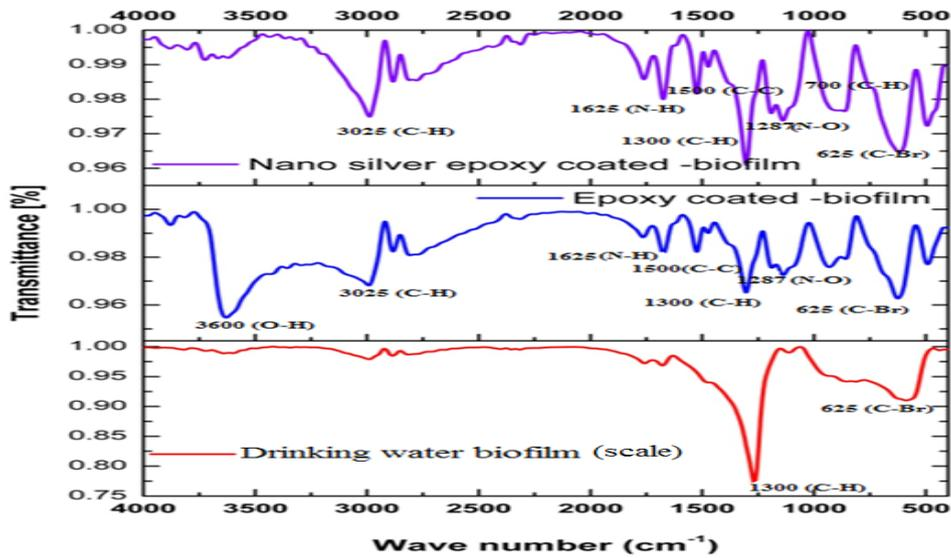
Fig. 4 FT-IR spectra of drinking water biofilm treated with Epoxy coating and Epoxy coated with silver nanoparticles
