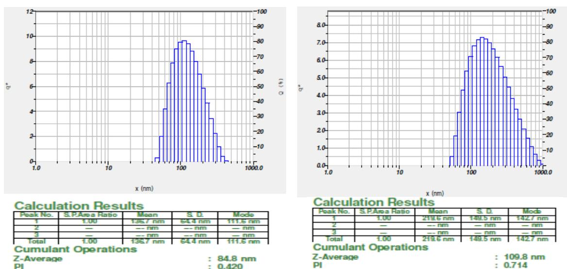
Fig. 6 Dynamic light scattering analysis (a) Particle size of *Alstonia scholaris* mediated synthesis of AgNPs (b) Particle size of epoxy coated *Alstonia scholaris* AgNPs
