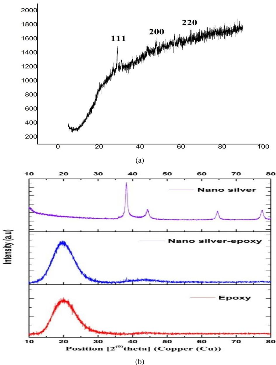
Fig. 5 XRD Patterns of (a) Nano silver, showing the typical face centered cubic crystal structure of the silver with predominant (111) face (b) Nano silver - epoxy
