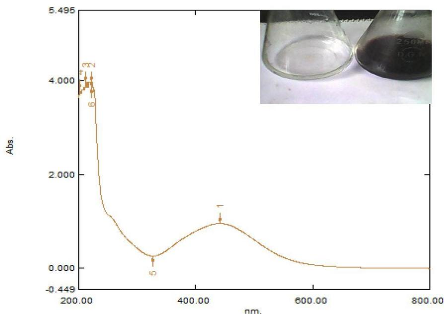
Fig. 2 UV-visible spectroscopic micrograph showing the localized surface plasmon resonance (LSPR) of Ag nanoparticles (420 nm) synthesized using *A. scholaris* bark extract
