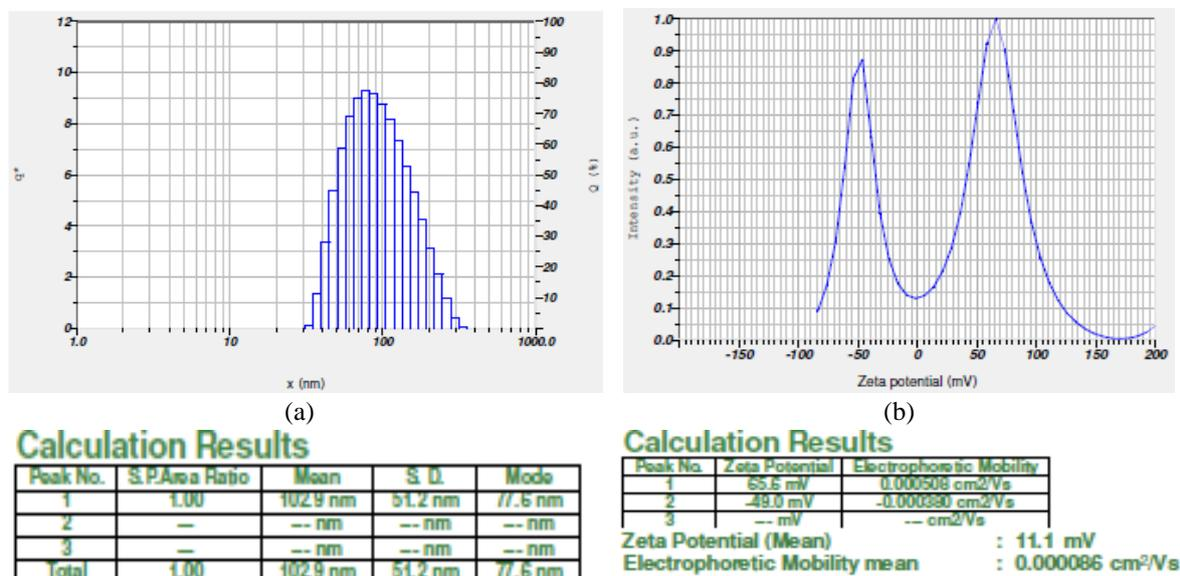
Fig. 6(a), (b) the histogram (size distribution) of silver nanoparticles (dynamic light scattering) and zeta potential (11.1 mV) of silver nanoparticles synthesized using *Luffa acutangula* leaf extract
