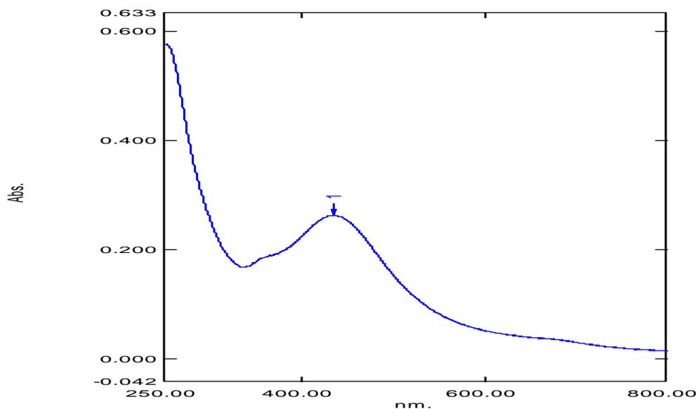
Fig. 3 Vis absorption spectrum of silver nanoparticles after 1 hour of reaction
