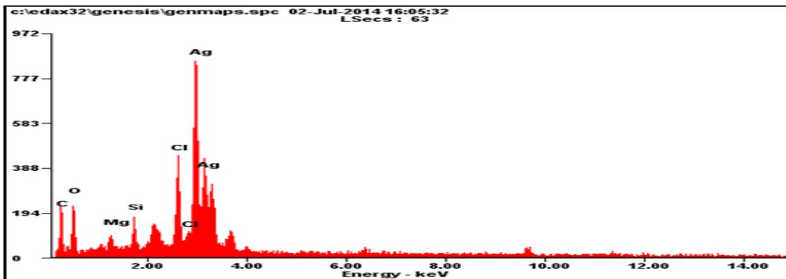
Fig. 8 Energy dispersion X-ray spectrum (EDS) micrograph of bio-synthesized AgNPs showing the elemental presence of Ag, C, O, Si and Mg
