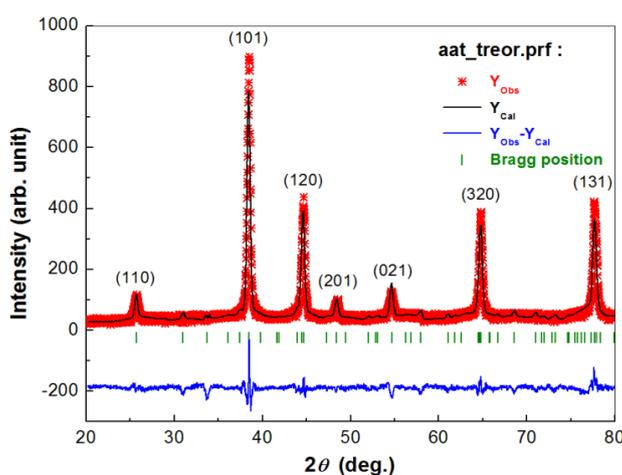
Fig. 1 Rietveld refined XRD pattern of nanocrystalline powder of  $Al_{0.5}Ag_{0.5}TiO_3$  in the space group  $P2/m(10)$ . Symbols represent observed data points and solid lines their Rietveld fit
