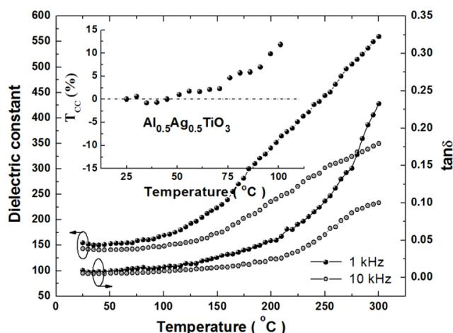
Fig. 6 Temperature dependence of dielectric constant and loss tangent of  $\text{Al}_{0.5}\text{Ag}_{0.5}\text{TiO}_3$  ceramic pellet at 1 kHz and 10 kHz. Inset: Variation of  $T_{CC}(\%)$  with temperature at 1 kHz
