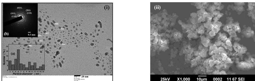
Fig. 3 (i) TEM image, particle size distribution (inset: a), SAED pattern (inset: b) and (ii) SEM image of nanocrystalline  $\text{Al}_{0.5}\text{Ag}_{0.5}\text{TiO}_3$  powder
