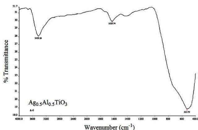
Fig. 4 FTIR spectrum of nanocrystalline  $\text{Al}_{0.5}\text{Ag}_{0.5}\text{TiO}_3$  powder
