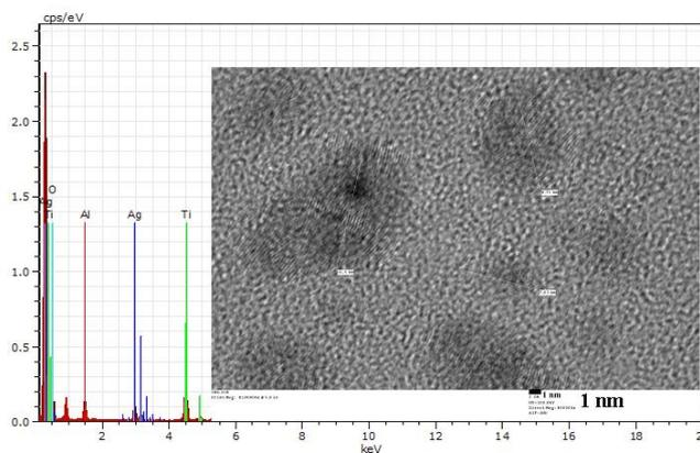
Fig. 2 EDX spectrum and HR-TEM image (inset) of nanocrystalline  $\text{Al}_{0.5}\text{Ag}_{0.5}\text{TiO}_3$  powder
