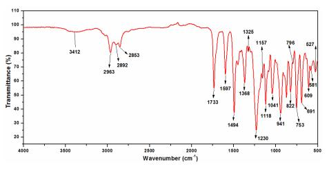
Fig. 6 FTIR of BPA aniline based benzoxazine monomer
