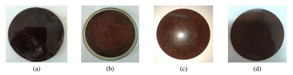
Fig. 1 Sawdust reinforced polybenzoxazine composites, (a) 20 wt% of SD, 80 wt% of PBZ; (b) 30 wt% of SD, 70 wt% of PBZ; (c) 40 wt% of SD, 60 wt% of PBZ; and (d) 45 wt% of SD, 55 wt% of PBZ
