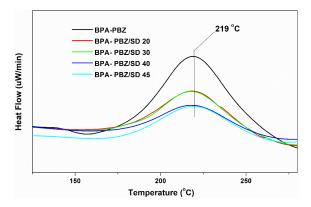
Fig. 4 DSC Thermograms of different compositions of BPA-PBZ/SD composites and their weight percentages
