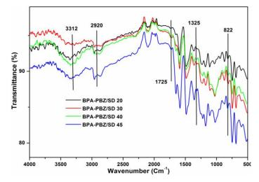
Fig. 10 FTIR Spectra of various weight ratios of sawdust reinforced polybenzoxazine composites
