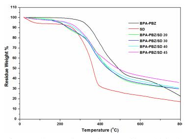
Fig. 2 TGA plots of BPA-PBZ/SD composites at various compositions and their values, PBZ, and SD
