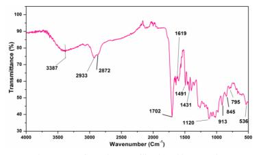
Fig. 7 FTIR of cured BPA aniline based benzoxazine
