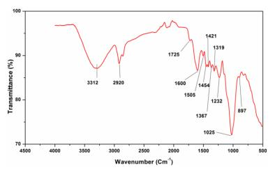
Fig. 8 FTIR spectra of raw sawdust
