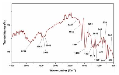
Fig. 9 FTIR of 20 wt% reinforced polybenzoxazine composite
