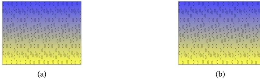
Fig. 3 Porosity models: (a) Evenly distributed porosities; (b) Unevenly distributed porosities
