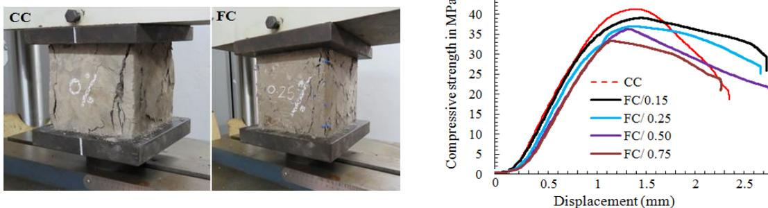
Fig. 4 Compressive strength test (a) Failure pattern; (b) Variation of strength with respect to fiber dosage
