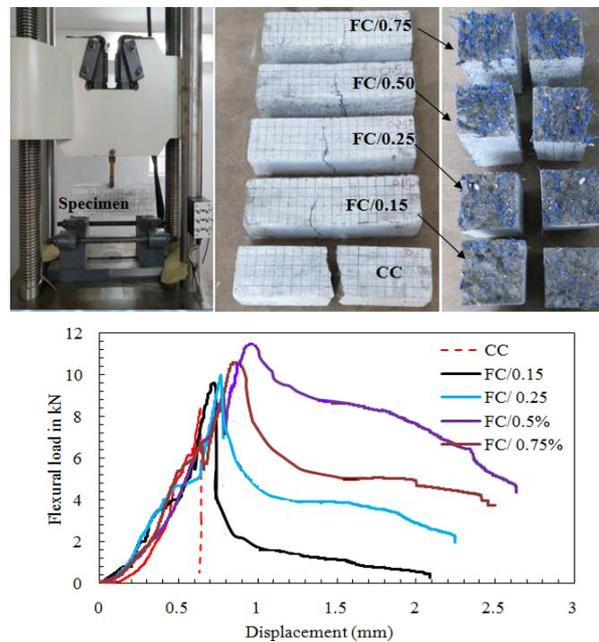
Fig. 6 Flexural strength test (a) test set-up, failure pattern and fiber distributions; (b) Variation of strength with respect to fiber dosage
