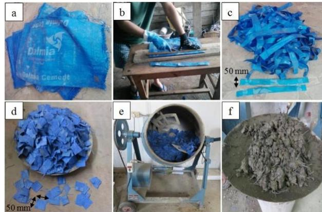
Fig. 2 Cutting process of PP fibers (a) PPCB; (b) Cutting of 50 mm strip; (c) Bunch of strips; (d) Fabric of 50 mm square size; (e) Mixing of small fabric with aggregate; (d) Discrete fiber formed after mixing
