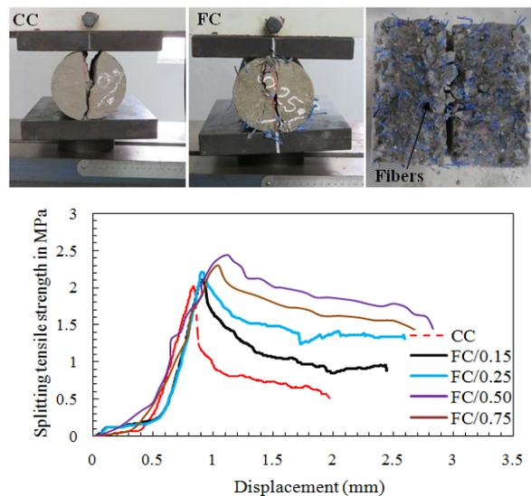
Fig. 5 Splitting tensile strength test (a) Failure pattern; (b) Variation of strength with respect to fiber dosage
