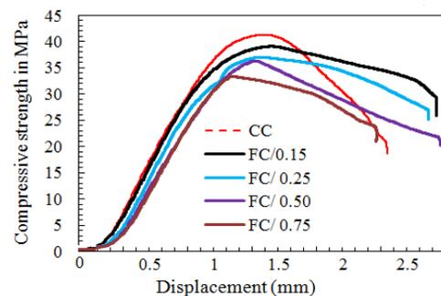
Fig. 4 Compressive strength test (a) Failure pattern; (b) Variation of strength with respect to fiber dosage
