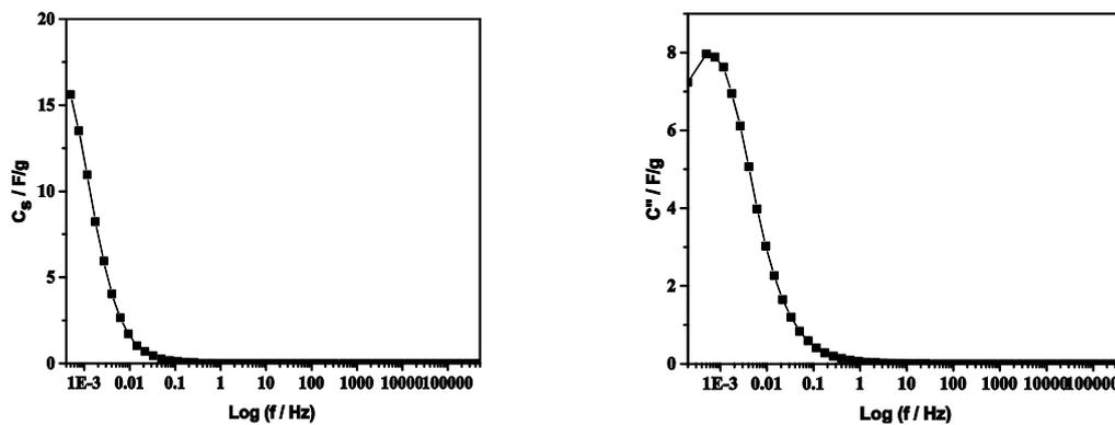
Fig. 2 (a) Variation of real part of capacitance with the frequency for an EDLC at room temperature; (b) variation of imaginary part of capacitance with the frequency for an EDLC at room temperature
