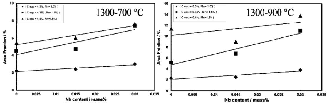
Fig. 5 The effect of Nb on the area fraction of MA at constant Mn (1.5%) after different heat cycles
