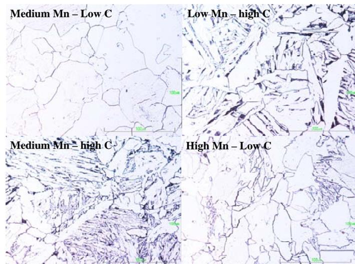
Fig. 1 The effect of variation in Mn and C within the same C equivalent on the microstructure at constant Nb (0.015%) after double cycle of 1300°C followed by 700°C
