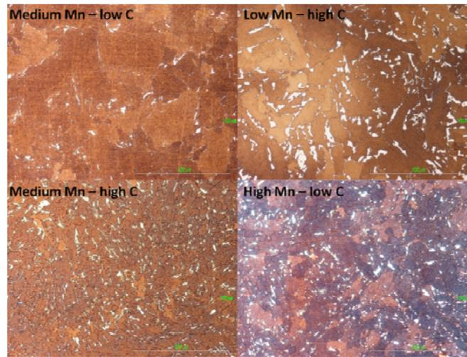
Fig. 4 The effect of variation in Mn and C within the same C equivalent on the microstructure at constant Nb (0.015%) after double cycle of 1300°C followed by 900°C
