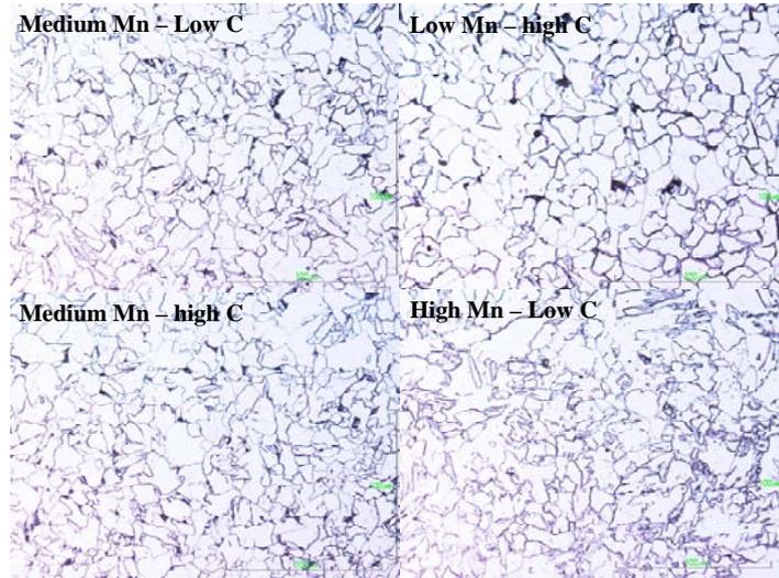
Fig. 2 The effect of variation in Mn and C within the same C equivalent on the microstructure at constant Nb (0.015%) after double cycle of 1300°C followed by 900°C
