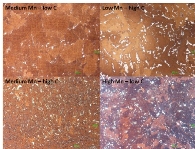
Fig. 3 The effect of variation in Mn and C within the same C equivalent on the microstructure at constant Nb content of 0.015% after double cycle of 1300°C followed by 700°C
