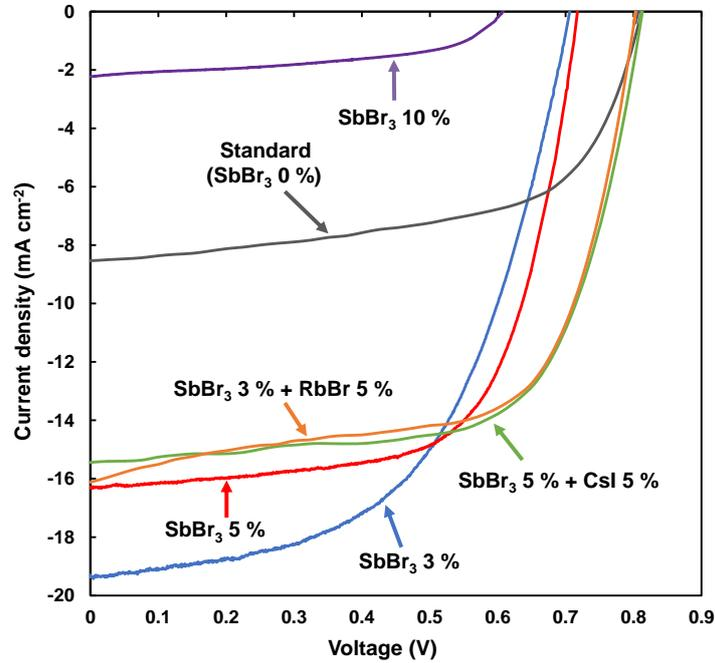
Fig. 2  $J$ - $V$  characteristic of present photovoltaic devices
