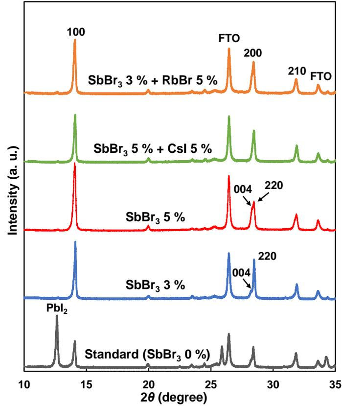
Fig. 4 XRD patterns of the present perovskite photovoltaic devices
