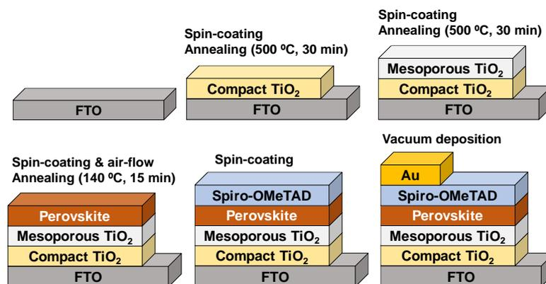
Fig. 1 Schematic illustration for the fabrication process of the present photovoltaic devices
