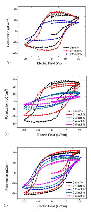
Fig. 6 Polarisation hysteresis curves for (a) KNN-BiZ ceramics, (b) KNNLT-BiZ ceramics (c) KNNLST-BiZ ceramics measured at room temperature with a 20 kV/cm electric field. The remnant polarization ( $P_r$ ) and coercive field ( $E_c$ ) values are shown in Table 2
