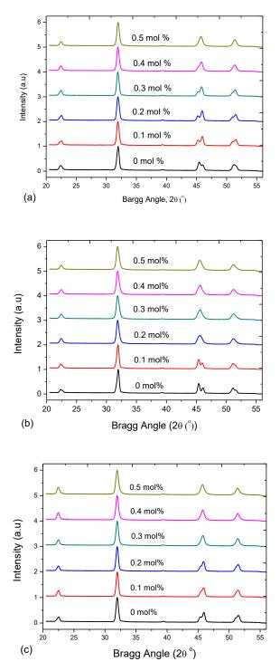
Fig. 2 X-ray diffraction patterns for (a) KNN-BiZ ceramic compositions, (b) KNNLT-BiZ ceramic compositions and (c) KNNLST-BiZ ceramics doped with  $Bi_4Zr_3O_{12}$
