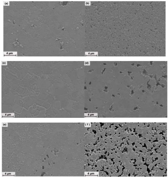
Fig. 3 Scanning Electron Microscope (SEM) images of the polished surfaces of (a) undoped KNN sintered at 1080°C. (b) KNN 0.5 mol% BiZ sintered at 1100°C (c) KNNLT 0 mol% BiZ sintered at 1100 °C (d) KNNLT 0.25 mol% BiZ sintered at 1100°C (e) KNNLST 0 mol% BiZ sintered at 1080°C (f) KNNLST 0.25 mol% BiZ sintered at 1090°C
