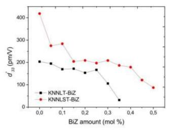
Fig. 7 Graph of piezoelectric charge coefficient from high signal measurements for KNNLT and KNNLST compositions as a function of the amount of BiZ modification
