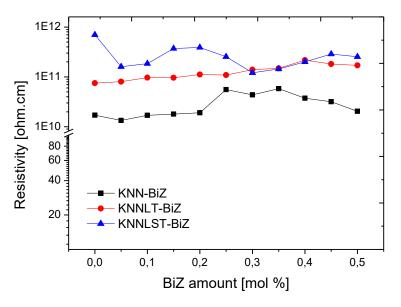
Fig. 5 Resistivity values for KNN, KNNLT and KNNLST compositions doped with different amounts of BiZ and measured at room temperature
