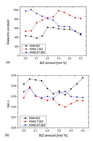
Fig. 4 (a) Dielectric constant values and (b) dielectric loss for KNN, KNNLT and KNNLST samples modified with different amounts of BiZ. The measurement was made at room temperature and at 1 KHz
