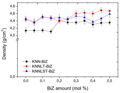
Fig. 1 Density values for KNN, KNNLT and KNNLST ceramics doped with  $Bi_4Zr_3O_{12}$ . The samples were sintered in air at temperatures ranging from 1080°C to 1130°C for 1 h
