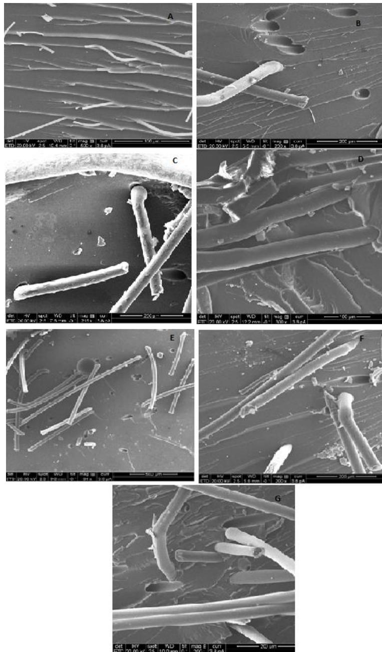
Fig. 10 Scanning electron micrographs of (A) Neat Epoxy, (B) E11, (C) E22, (D) E33, (E) E55, (F) E77 and (G) E50
