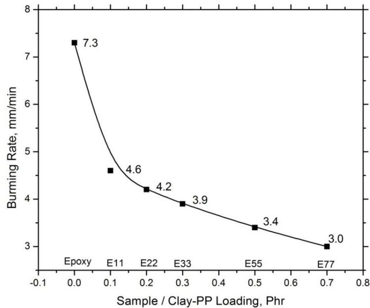
Fig. 9 Burning rates of epoxy-PP short fiber-clay composites
