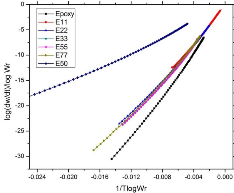
Fig. 8 Freeman-Carroll kinetic plot to find  $E_a$  of epoxy-PP short fibers -clay composites
