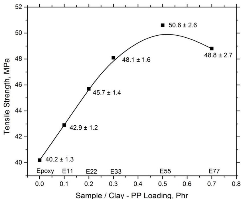
Fig. 2 Tensile strengths of epoxy-PP short fibers -clay composites
