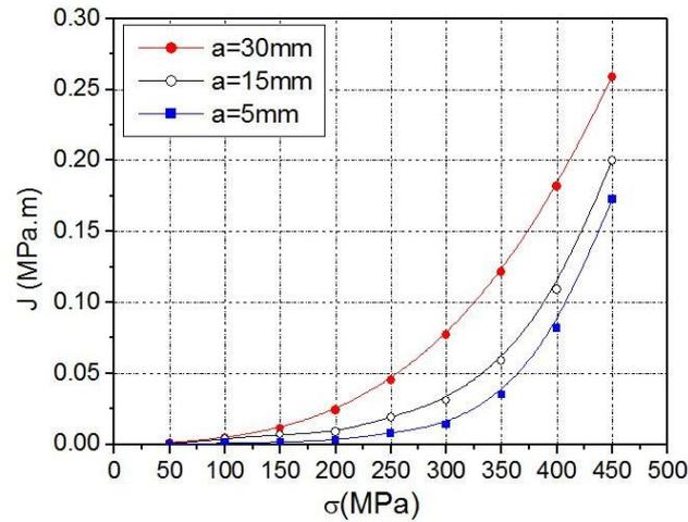
Fig. 9 Variation of the  $J$  integral according to the stress for different crack length,  $b=20$  mm,  $h=250$  mm
