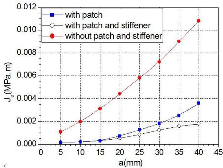
Fig. 5 Variation of the J integral according to the crack length for the cases with and without patch and stiffener
