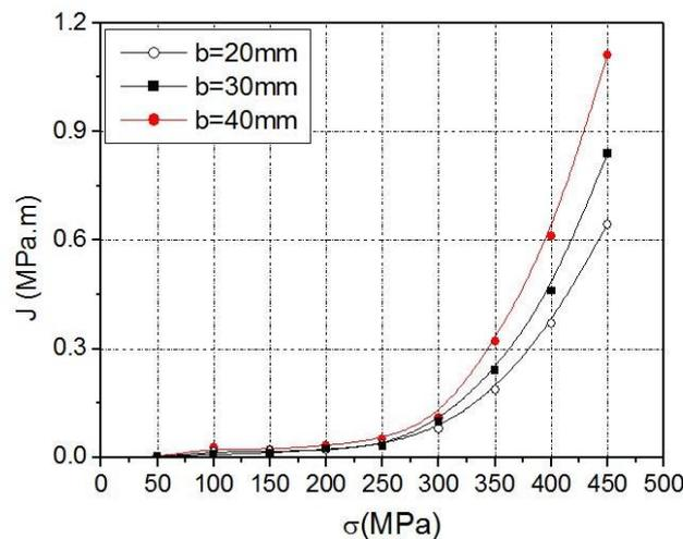
Fig. 10 Variation of the  $J$  integral according to the stress for different value of inter-distance ( $b$ ),  $h=250$  mm,  $a=45$  mm
