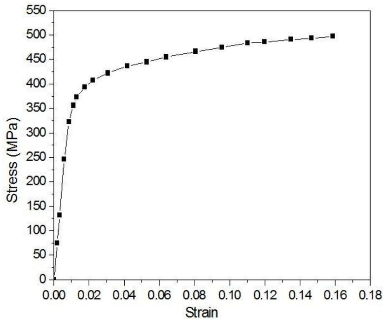
Fig. 2 Stress-strain curves for aluminum 2024-T3
