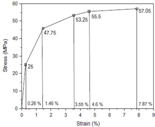
Fig. 3 Multi-linear stress-strain curve of the FM 73 epoxy adhesive (Ban *et al.* 2008)
