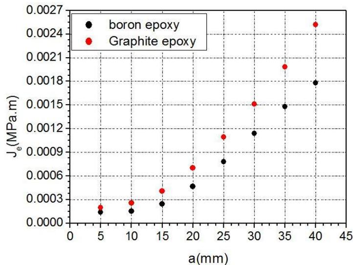
Fig. 7 the variation of the  $J$  integral according to the cracks for two different properties of the patch
