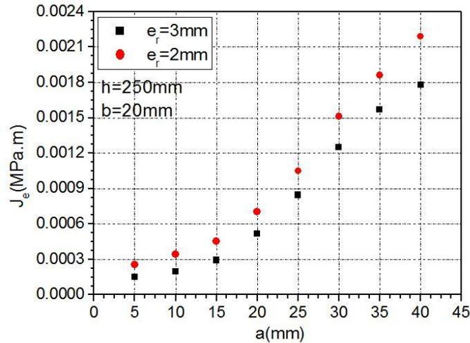
Fig. 6 Variation of the  $J$  integral according to the patch thickness for different cracks
