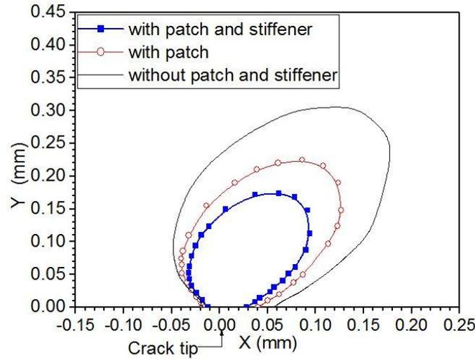
Fig. 8 Contour of the plastic zone for the cases with and without patch
