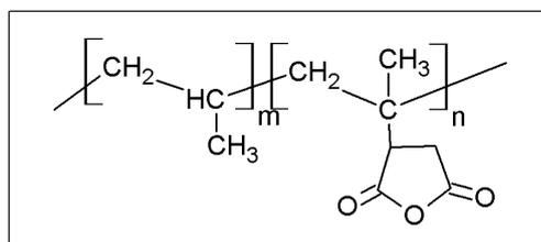
Fig. 1 Chemical structure of MAPP
