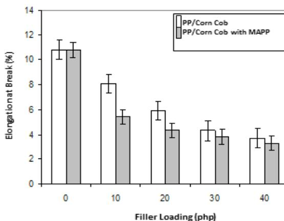
Fig. 4 The effect of filler loading on elongation at break of uncompatibilized and compatibilized PP/CC biocomposites
