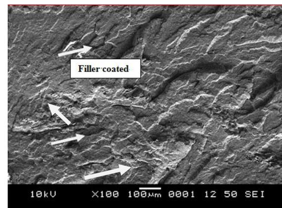
Fig. 9 The SEM micrograph of tensile fracture surface of compatibilized biocomposite (40 php corn cob)
