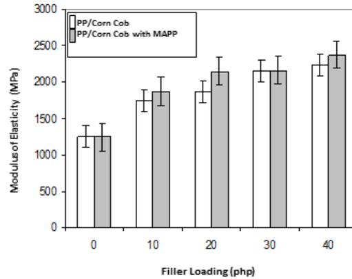
Fig. 5 The effect of filler loading on modulus of elasticity of uncompatibilized and compatibilized PP/CC biocomposites
