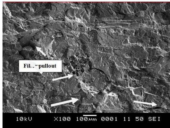
Fig. 6 The SEM micrograph of tensile fracture surface of uncompatibilized biocomposite (20 php corn cob)
