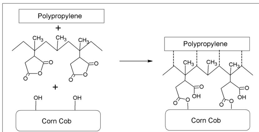
Fig. 3 Proposed schematic reaction between PP/corn cob biocomposite and MAPP
