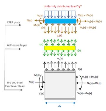
Fig. 2 Forces in infinitesimal element of a soffit-CFRP plated steel cantilever beam
