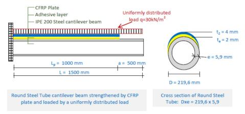
Fig. 4 Round Steel tube cantilever beam strengthened by CFRP plate and loaded by a uniformly distributed load
