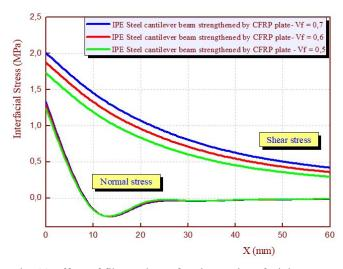
Fig. 11 Effect of fiber volume fraction on interfacial stresses
