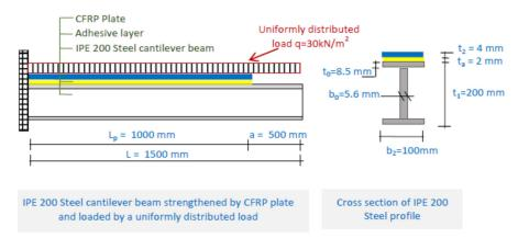
Fig. 3 IPE 200 Steel cantilever beam strengthened by CFRP plate and loaded by a uniformly distributed load
