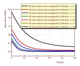
Fig. 9 Effect of the fiber orientation on the interfacial shear stresses for steel cantilever beam with a bonded CFRP soffit plate
