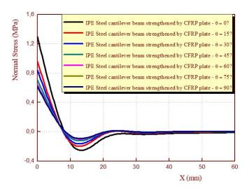
Fig. 10 Effect of the fiber oriejntation on the interfacial normal stresses for steel cantilever beam with a bonded CFRP soffit plate
