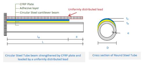
Fig. 1 Structure configuration of a circular steel beam strengthened by CFRP plate and loaded by a uniformly distributed load
