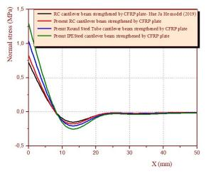
Fig. 6 Comparison of interfacial normal stress for CFRP-plated Steel cantilever beam with the analytical results
