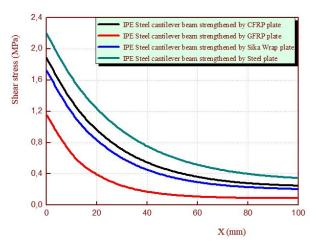
Fig. 7 Effect of plate stiffness on interfacial shear stresses
