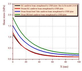
Fig. 5 Comparison of interfacial shear stress for CFRP-plated Steel cantilever beam with the analytical results
