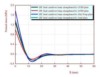
Fig. 8 Effect of plate stiffness on interfacial normal stresses
