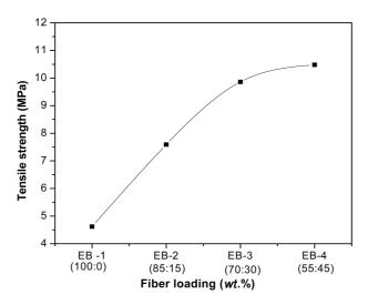
Fig. 2(a) Effect of fiber loading on tensile strength of composites
