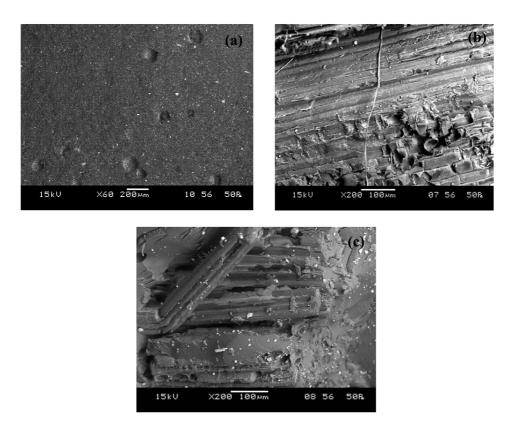
Fig. 5 Scanning electron micrographs of bamboo fiber reinforced epoxy composite specimens before and after tensile testing
