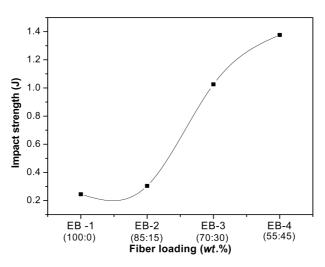
Fig. 4a Effect of fiber loading on impact strength of composites
