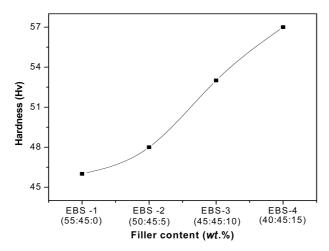
Fig. 1(b) Effect of filler content on hardness of composites
