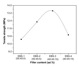
Fig. 2(b) Effect of filler content on tensile strength of composites
