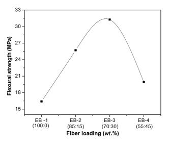
Fig. 3a Effect of fiber loading on flexural strength of composites
