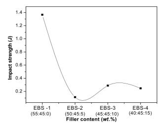
Fig. 4b Effect of filler content on impact strength of composites
