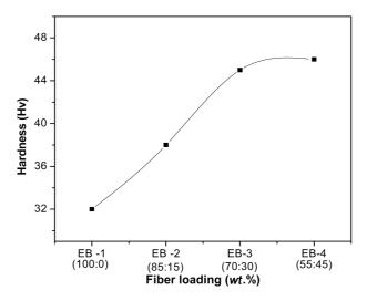
Fig. 1(a) Effect of fiber loading on hardness of composites
