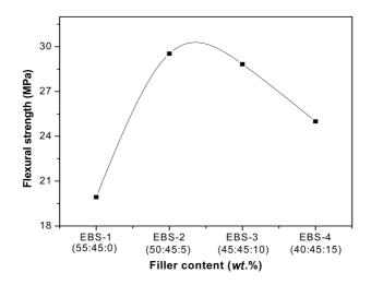
Fig. 3b Effect of filler content on flexural strength of composites
