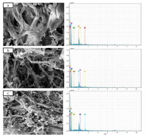
Fig. 5 SEM micrographs and EDX profiles for (a) Fungus (T. versicolor), (b) EBP loaded fungus and (c) OBH loaded fungus (10000 KX)
