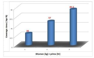
Fig. 5 Bitumen with different proportion of primer coverage
