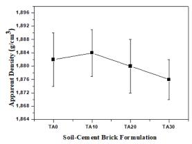
Fig. 4 Apparent density of the soil-cement bricks
