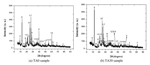
Fig. 1 XRD patterns of the cured soil-cement bricks. 1-quartz, 2-kaolinite, 3-illite/mica, 4-gibbsite, 5-goethite, 6-ettringite, 7-calcium silicate hydrate, 8-portlandite, 9-potassium carbonate, 10-cristobalite and 11-hematite
