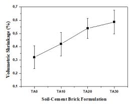
Fig. 3 Volumetric shrinkage of the soil-cement bricks
