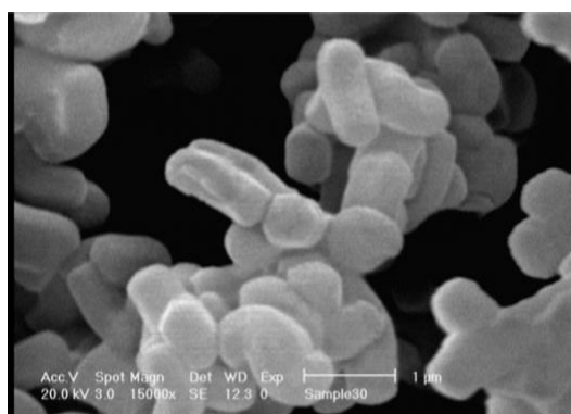
Fig. 5 SEM image calcined of hexagonal SBA-15 (the magnification \times 15000)
