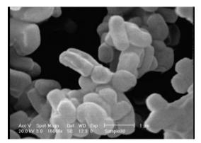
Fig. 5 SEM image calcined of hexagonal SBA-15 (the magnification×15000)
