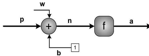
Fig. 2 An artificial neuron schematic (Asadollahfardi 2015)
