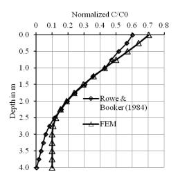
Fig. 1 Validation of FEM results with Rowe and Booker (1984) Table 2 Material Properties from Sharma *et al.* (2014)
