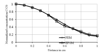
Fig. 3 Validation of EFGM results with FEM results in heterogeneous media
