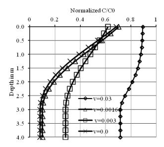
Fig. 6 Effect of change of advective of velocity of top layer
