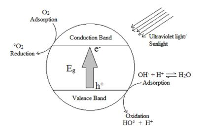
Fig. 1 Schematic diagram of photoexcitation of semiconductor by UV/solar irradiation
