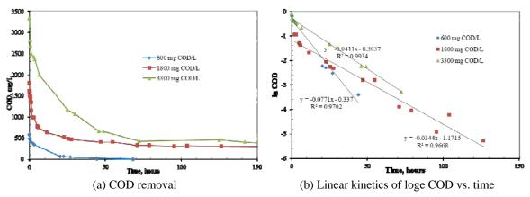
Fig. 4 Kinetics of COD removal from artificial olive waste
