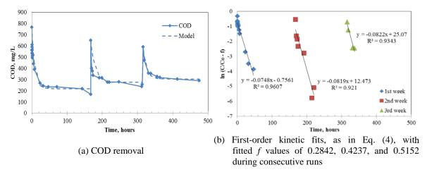
Fig. 5 COD removal kinetics for blended olive mill waste using the P/TF system
