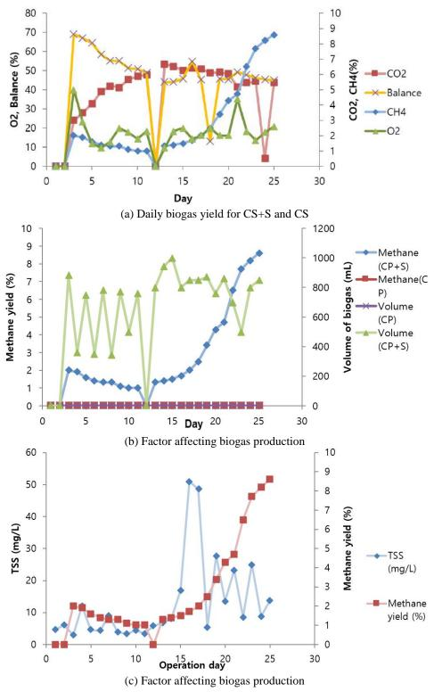
Fig. 4 Graph of daily biogas yield for CS+S and CS (a), factors affecting biogas production (b), and (c)
