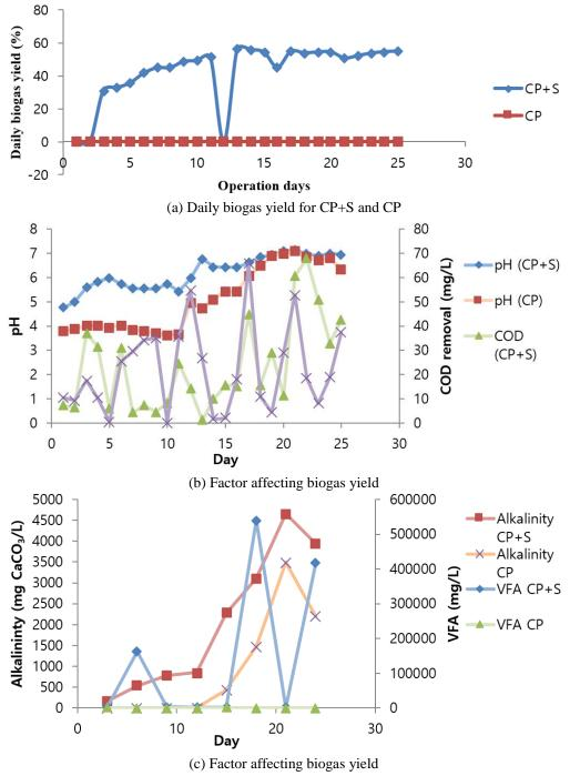
Fig. 3 Graph of daily biogas yield for CP+S and CP (a), factors affecting biogas yield (b) and (c)
