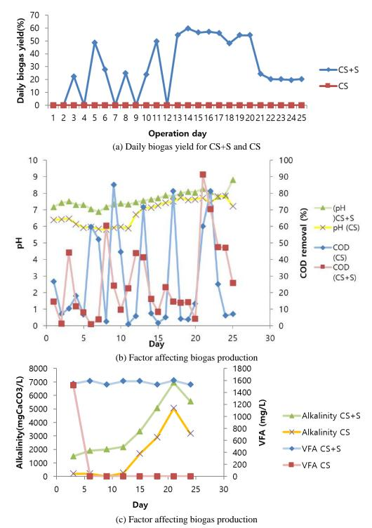
Fig. 4 Graph of daily biogas yield for CS+S and CS (a), factors affecting biogas production (b) and (c)
