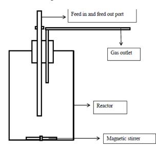
Fig. 2 CSTR schematic layout
