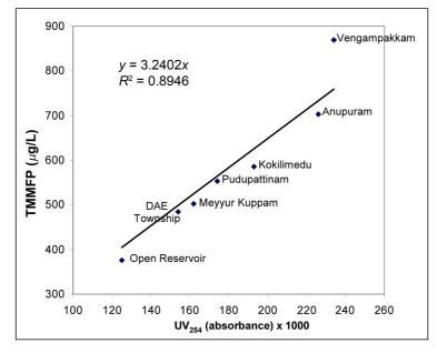
Fig. 3 Dependence of THMFP on unsaturated organics (UV<sub>254</sub>)
