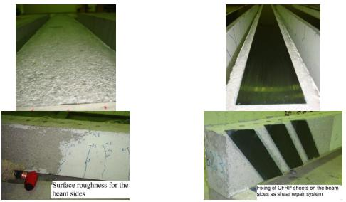
Fig. 3 Surface preparation and CFRP fixing for flexural and shear
