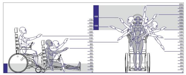
Fig. 6 Ergonomic scheme of the wheelchair
