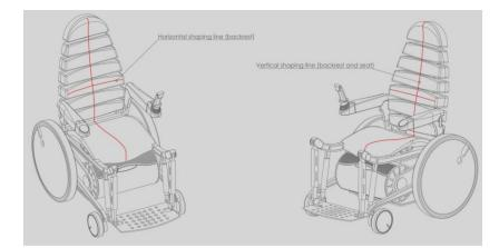
Fig. 5 Shaping lines of the backrest and seat with parameters provided by B. Akerblom
