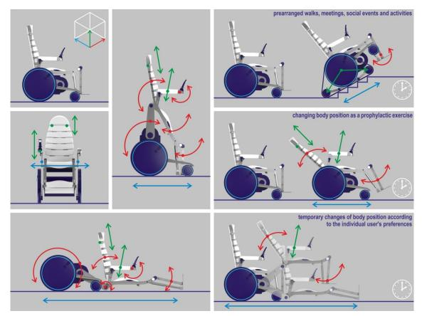
Fig. 9 Transformation of the wheelchair into different positions and within a specified period of time
