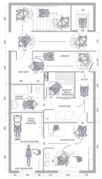
Fig. 11 Graphical analysis of optimal model of transportation in medical center
