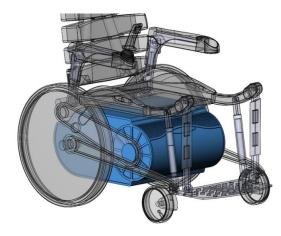
Fig. 8 The energy block of the wheelchair
