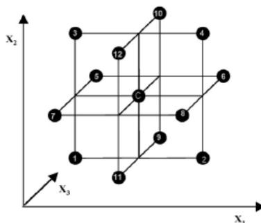
Fig. 2 Three-level full factorial design for three factors experiment
