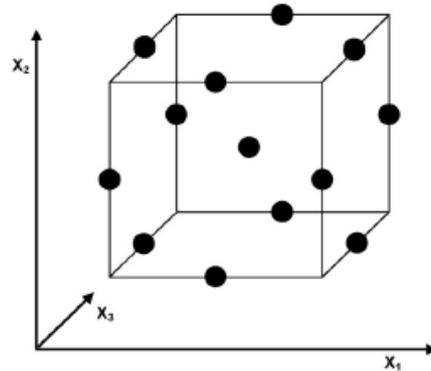
Fig. 4 Box–Behnken design for a three-factor experiment
