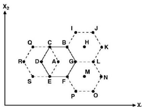
Fig. 1 Hexagonal Doehlert two factors design with three possible displacements in the experimental space
