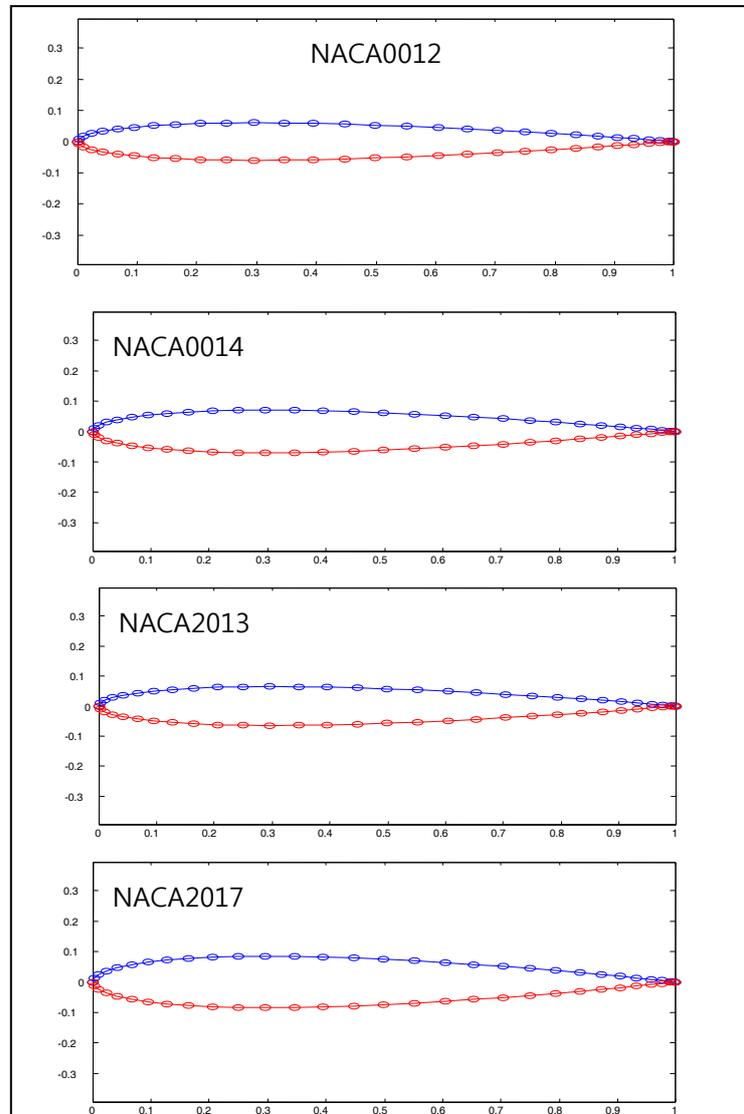
Fig. 5 Generated airfoil profiles
