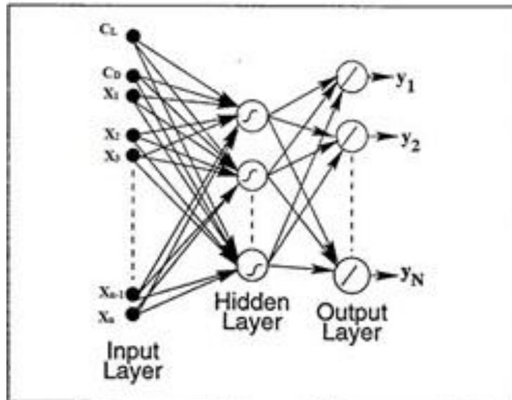
Fig. 2 Neural network trained to predict surface Y-coordinates of Airfoil
