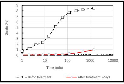
Fig. 6 Swelling Potential curves Before and After Treatment 7 days
