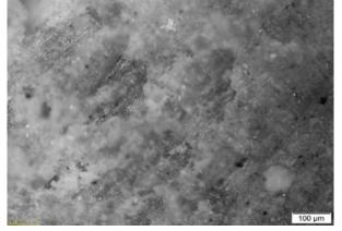
Fig. 8c Scanning electron micrograph of treatment lime 6% after 28 days
