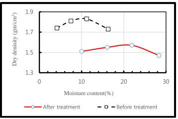
Fig.4 Compaction curves Before and After Treatment
