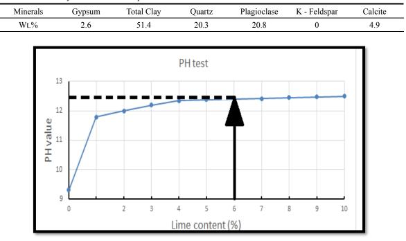
Fig. 2 Relationship between pH values and Lime content (%) to determine the optimum lime content of an expansive shell
