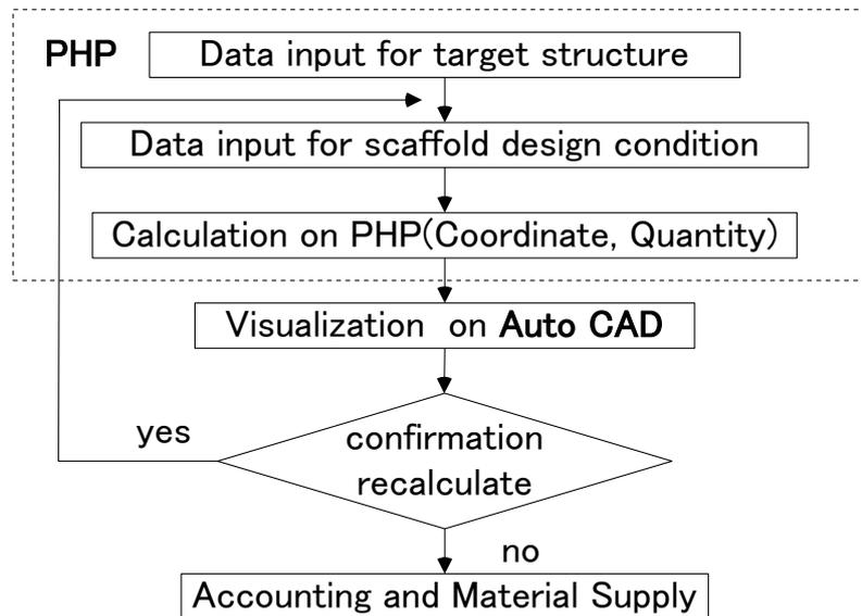
Fig. 1 Calculating and evaluating system
