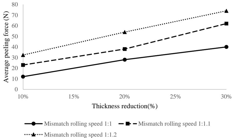
Fig. 8 Effect of mismatch speed ratio on the average peeling strength of samples
