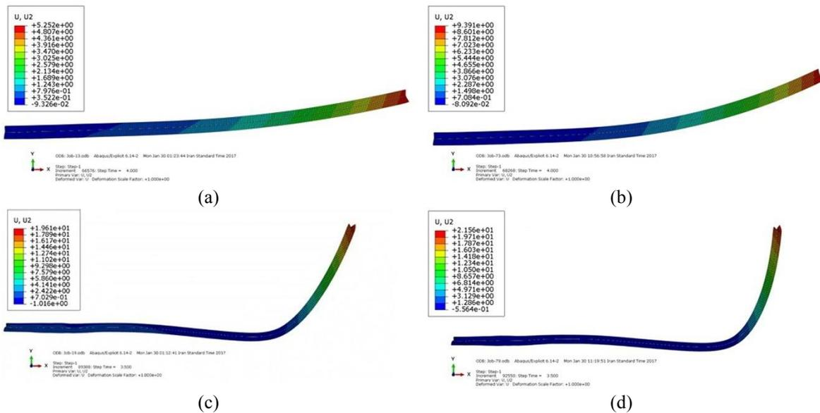
Fig. 5 Maximum vertical strain exerted on the bimetals strips with. (a, c) 1:1 and (b, d) 1:1.2
