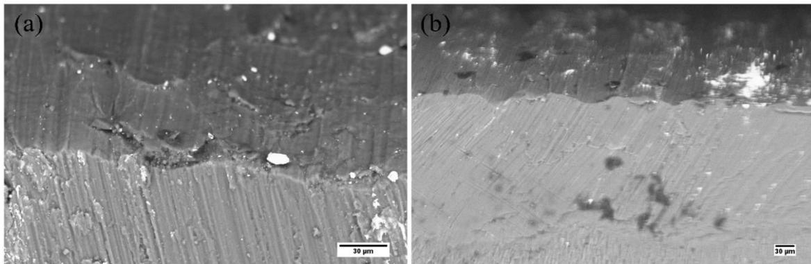
Fig. 7 SEM microstructure of as-rolled clad sheet with different mismatch speed ratios (a) 1:1 and (b) 1:1.2
