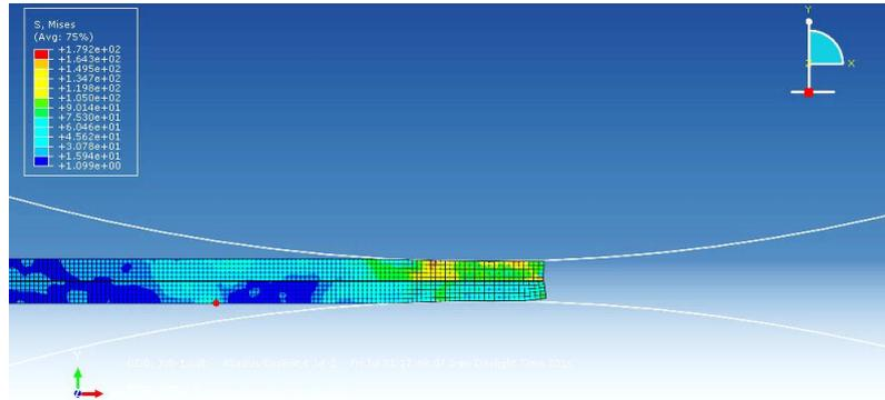
Fig. 4 Asymmetric rolling process of bimetals Al/Cu laminates
