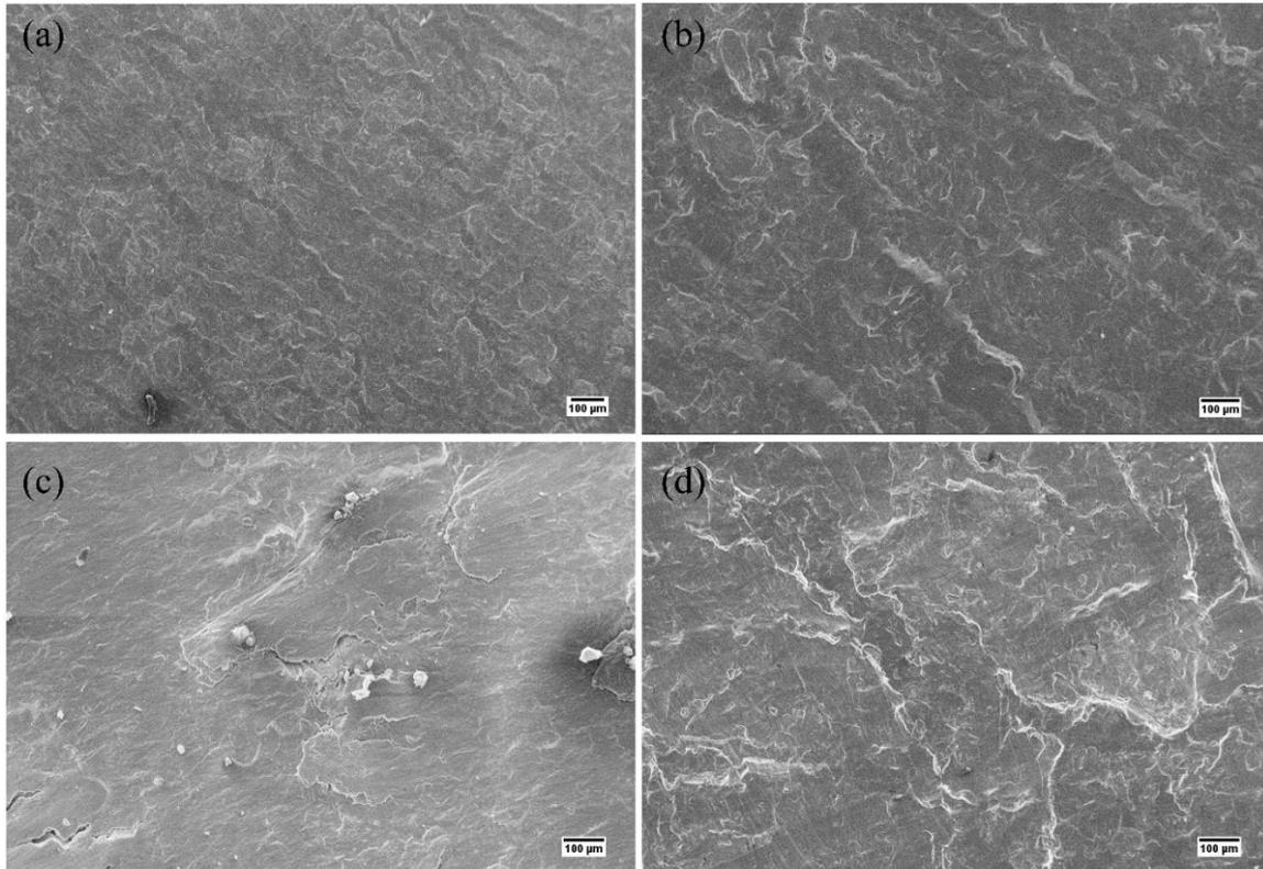
Fig. 9 SEM microstructure of peeled surface of samples with thickness reduction ratios (a, b) 10% and (c, d) 30%. Also, with different mismatch ratios as (a) 1:1, (b) 1:1.2, (c) 1:1 and (d) 1:1.2
