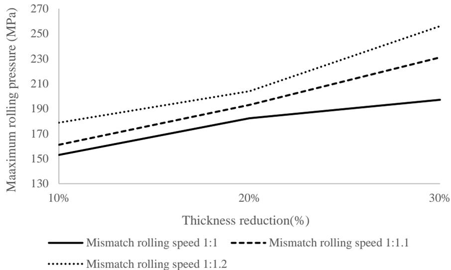
Fig. 6 Maximum stress exerted on the bimetal strips with different mismatch speed ratios
