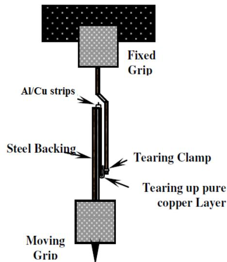
Fig. 2 Schematic illustration of the peeling test fixture
