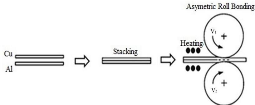
Fig. 1 Schematic diagram of asymmetrical RB process
