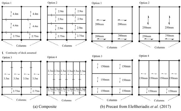
Fig. 3 Framing arrangements for the tested building as examined by the practicing structural engineers
