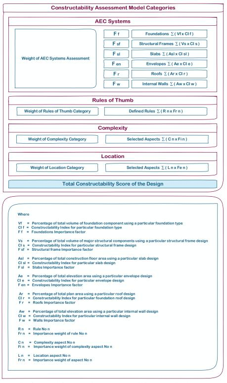
Fig. 5 Equation framework for calculating the constructability score using the proposed model
