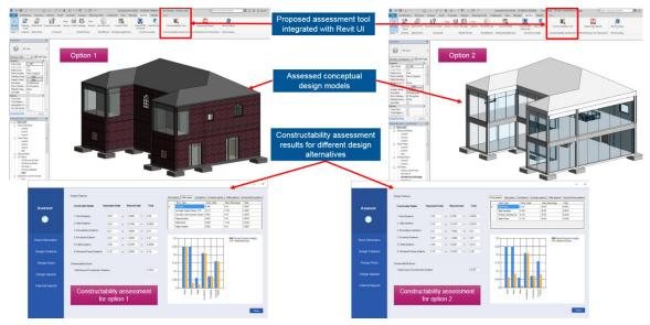
Fig. 8 Constructability scores of design alternatives
