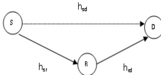
Fig. 2 Example network for cooperative transmission
